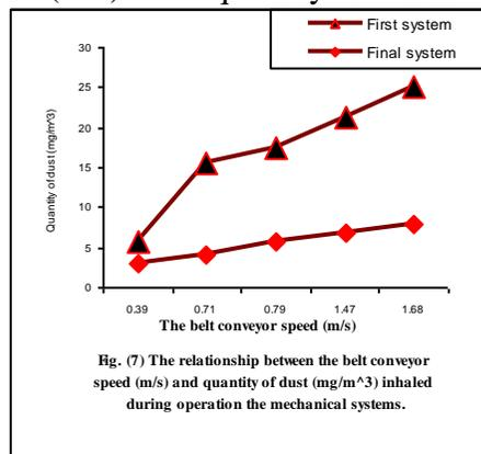
Fig. (7) The relationship between the belt conveyor speed (m/s) and quantity of dust (mg/m<sup>3</sup>) inhaled during operation the mechanical systems.
