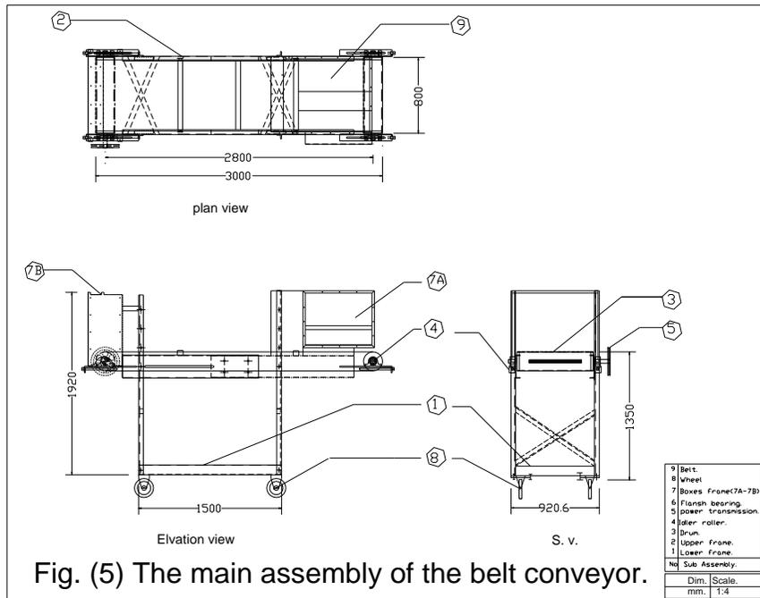
Fig. (5) The main assembly of the belt conveyor.
