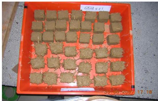
**Fig. (1): Samples prepared for drying test and water absorption.**
