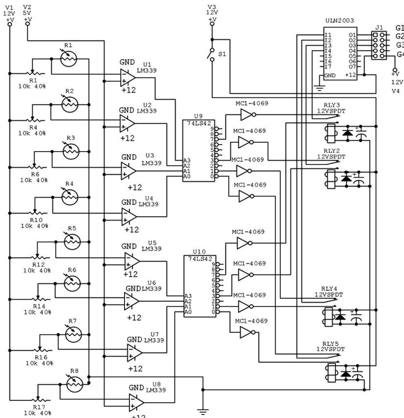
Fig(6) Photoresistor circuit
