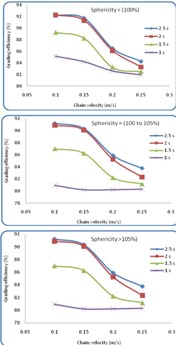
Fig. (8): Effect of conveyor chain velocity on the grading efficiency at different values of stopping time and sphericity percentage for onion.
