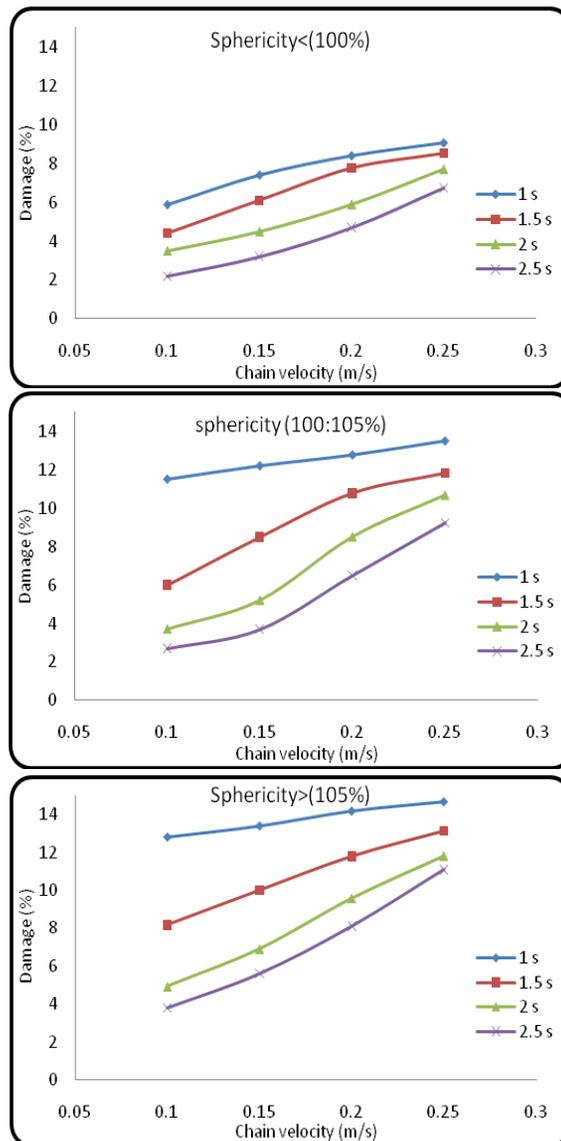
Fig. (9): Effect of chain velocity on damage percentage efficiency at different value of stopping time and sphericity percentage for onion.
