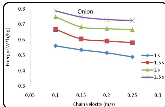
Fig.(10): Effect of conveyor chain velocity and stopping time on energy required for grading prototype .
