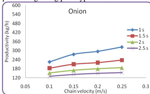
Fig.(11): Effect of conveyor chain velocity and stopping time on productivity of grading prototype.
