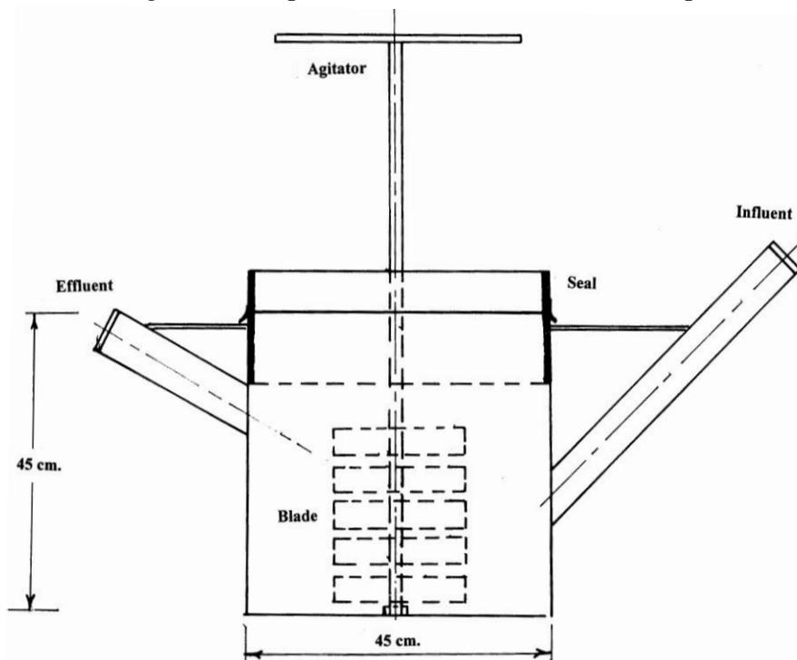
**Fig.(1): The used digester, (Drawn to scale).**
