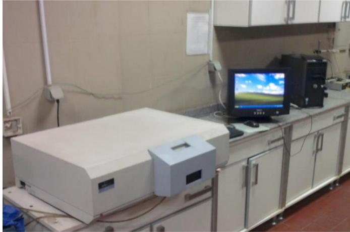
a) Plate of luminescence spectrometer
