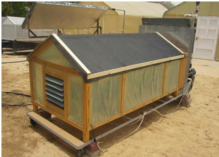
**Fig. (1): Experimental gable-even-span greenhouse**
