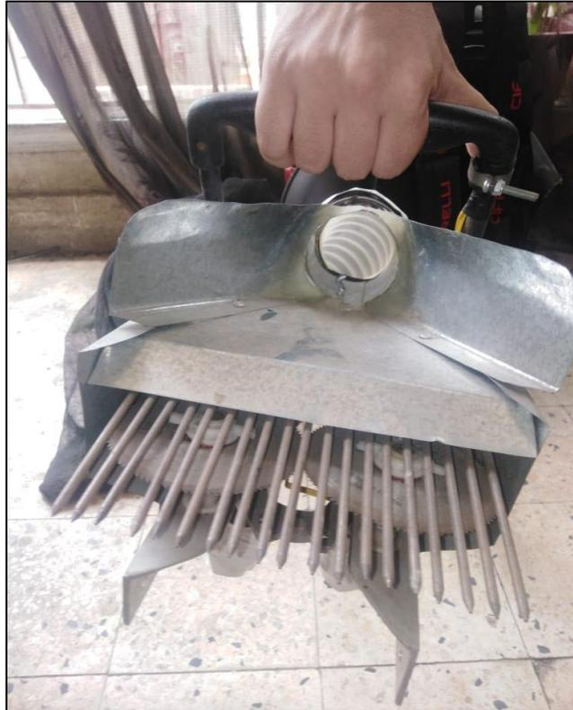
**Fig. (4): The cutting head and the collecting housing.**
