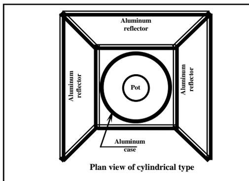
Figure (2) Plan view of aluminum cooker
