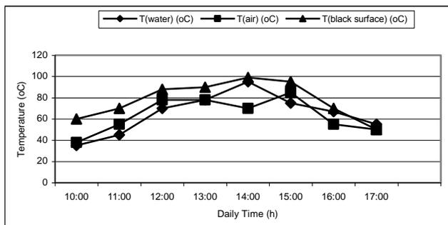
Figures (4): Effect of the Solar Radiation and the Daily Time on the Cooker Temperatures without load for aluminum box cooker in the 2<sup>nd</sup> of August 2011
