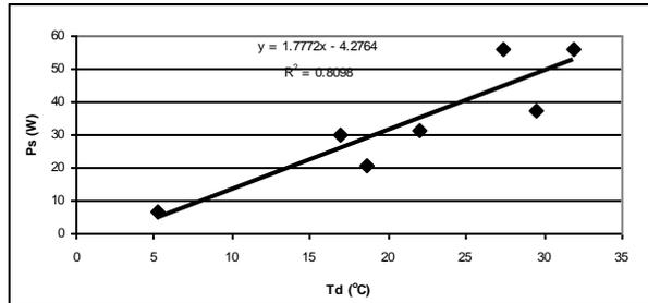
Figures (10): The standardized cooking power as a function of temperature difference ( $T_w-T_{amb}$ ) for aluminum box with 0.5 kg of water.
