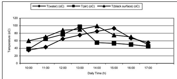
Figures (6): Effect of Cooker Type on the Cooker Temperatures for aluminum box with 1.0 kg of water
