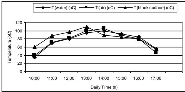
Figures (5): Effect of Cooker Type on the Cooker Temperatures for carton box with 1.0 kg of water
