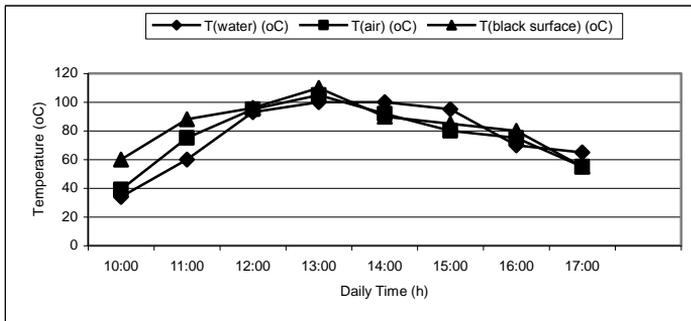
Figures (3): Effect of the Solar Radiation and the Daily Time on the Cooker Temperatures without load for carton box cooker in the 2<sup>nd</sup> of August 2011
