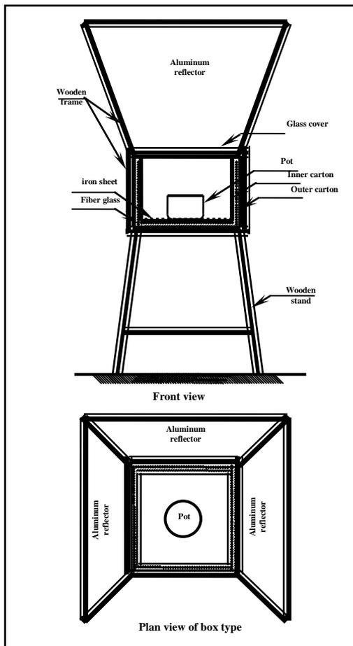
Figure (1) Front and plan view of carton cooker
