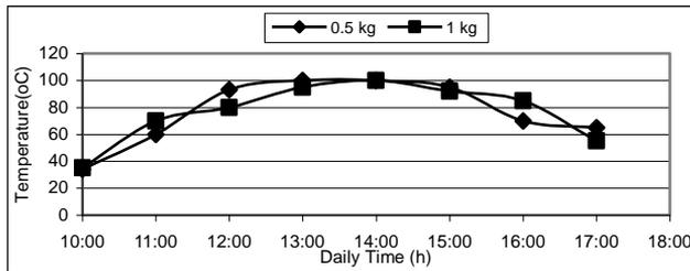
Figure (7): Effect of Load on the Cooker Temperatures for carton box
