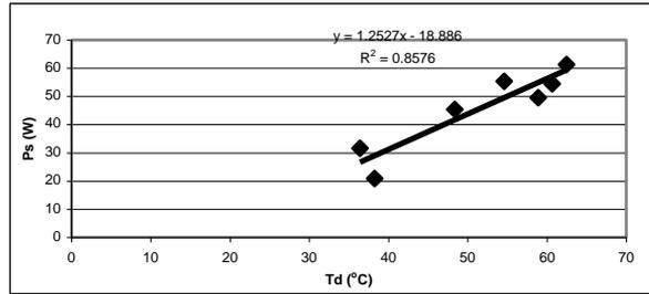
Figures (9): The standardized cooking power as a function of temperature difference ( $T_w-T_{amb}$ ) for carton box with 1 kg of water.
