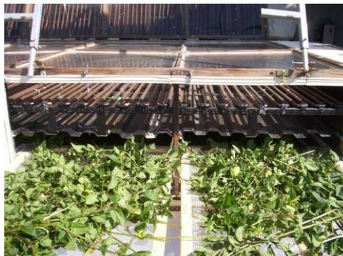
Fig. 4. Fresh Peppermint put over tray to dry in the solar dryer
