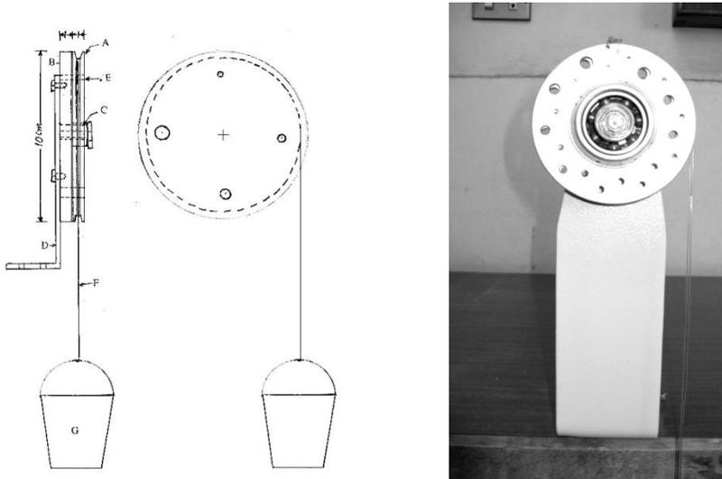
Figure (1): Static Shear Cell Apparatus. (A-Moving Disc B- Fixed Disc C- Ball Bearing D- Holder E- Hole F- Rope G- Water Bucket)
