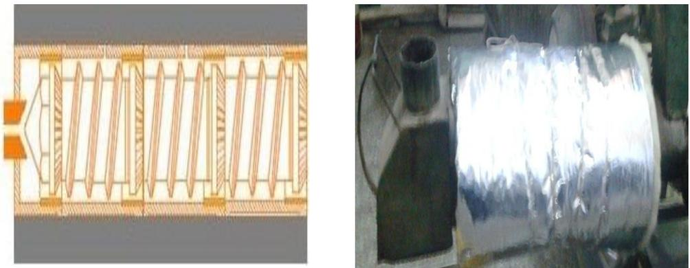
**Fig .3. Applied the critical radius of insulation on the extruder's barrel.**
