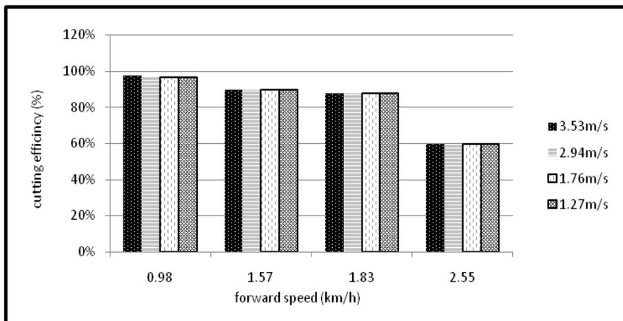
Fig. (9): The relation between cutting efficiency and forward speed for the modified mower
