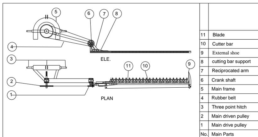
Fig. (1): The components of the original mower
