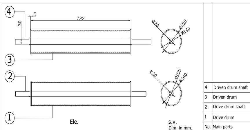
Fig. (2): The dimensions of the drive and driven drums
