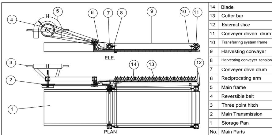
Fig (4): The mower after development
