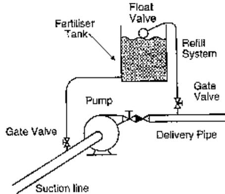
(b) Fertilizer injection with suction pipe of irrigation.
