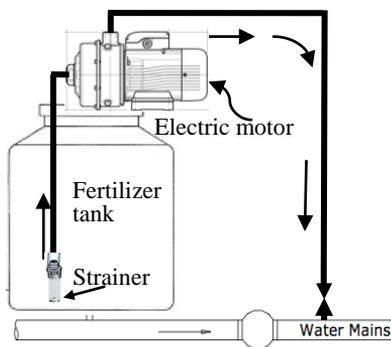
(c) Separate electric centrifugal injection pump (1.13 kW).
