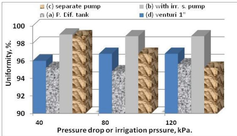
Fig. 4: Effect of pressure drop or irrigation pressure on injection rate uniformity for different chemical injection equipment.
