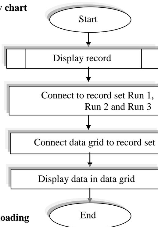
**Fig 2. Flow chart for data loading**
