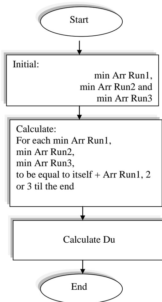
**Fig4. Flow chart for calculating distribution uniformity (Du)**
