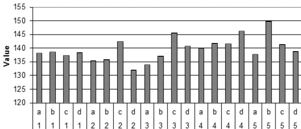
Figure 8. Average of the green and red values (digital numbers) for the five soil types 1 (sand clay loam), 2 (clay loam), 3 (silty clay loam), 4 (sandy), and 5 (clayey) at the four moisture contents [air dried (a), FC (b), 1.5FC (c), and 2.0FC (d)] at 90-cm camera height.
