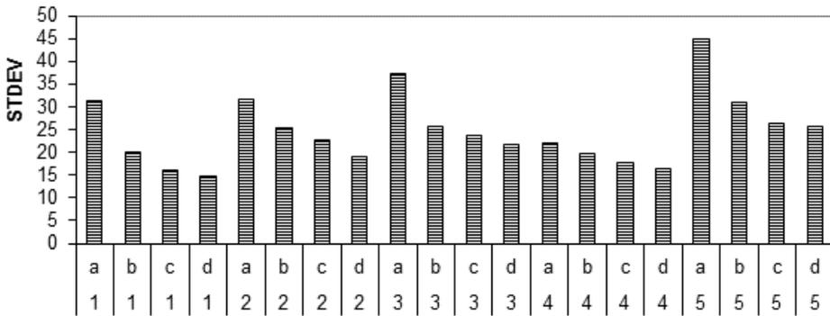
Figure 6. Average of the green and red standard deviations ( $ASD_{RG}$ ) for the five soil types 1 (sand clay loam), 2 (clay loam), 3 (silty clay loam), 4 (sandy), and 5 (clayey) at the four moisture contents [air dried (a), FC (b), 1.5FC (c), and 2.0FC (d)] at 60-cm camera height.
