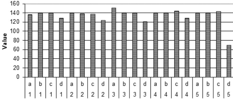
Figure 5. Average of the green and red values (digital numbers) for the five soil types 1, 2, 3, 4, and 5 at the 4 moisture contents (a, b, c, and d) at five soil types 1 (sand clay loam), 2 (clay loam), 3 (silty clay loam), 4 (sandy), and 5 (clayey) at the four moisture contents [air dried (a), FC (b), 1.5FC (c), and 2.0FC (d)] at 60-cm camera height.
