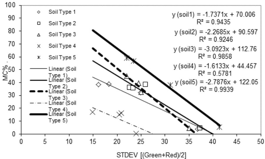
Figure 4. Moisture content (MC %) vs. average standard deviation of the green and red bands for the five soil types 1 (sand clay loam), 2 (clay loam), 3 (silty clay loam), 4 (sandy), and 5 (clayey) at the four moisture contents [air dried (a), FC (b), 1.5FC (c), and 2.0FC (d)] at 30-cm camera height.
