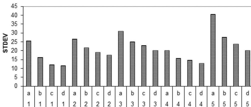
Figure 9. Average of the green and red standard deviations ( $ASD_{RG}$ ) for the five soil types 1 (sand clay loam), 2 (clay loam), 3 (silty clay loam), 4 (sandy), and 5 (clayey) at the four moisture contents [air dried (a), FC (b), 1.5FC (c), and 2.0FC (d)] at 90-cm camera height.
