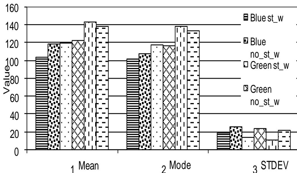
Figure 11. Mean value, mode and standard deviation (STDEV) (average of the three camera heights 30, 60 and 90 cm) for wet soil with standing vs. no standing water (sand clay loam) with blue, green and red channels.
