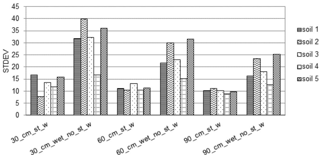
Figure 16. Using average standard deviation (STDEV of green and red channels) to distinguish between wet soil with standing water (st\_w) vs. no standing water (no\_st\_w) for soil types 1 (sand clay loam), 2 (clay loam), 3 (silty clay loam), 4 (sandy), and 5 (clayey).
