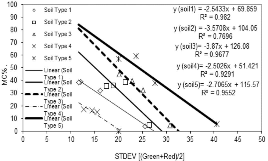
Figure 10. Moisture content (MC %) vs. average standard deviation of the green and red bands for the five soil types 1 (sand clay loam), 2 (clay loam), 3 (silty clay loam), 4 (sandy), and 5 (clayey) at the four moisture contents [air dried (a), FC (b), 1.5FC (c), and 2.0FC (d)] at 90-cm camera height.
