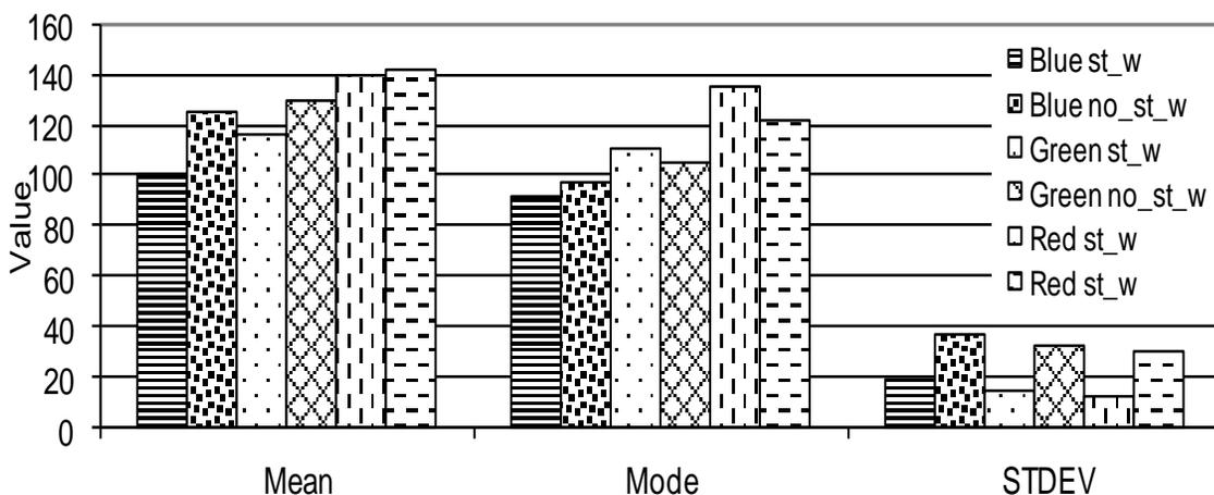
Figure 15. Mean value, mode and standard deviation (STDEV) (average of the three camera heights 30, 60 and 90 cm) for wet soil with standing vs. no standing water (clayey) with blue, green and red channels.
