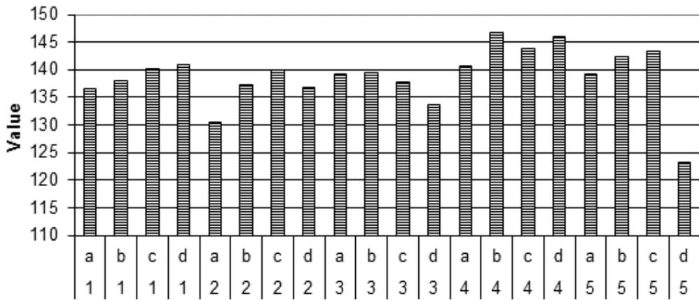
Figure 2. Average of the green and red values (digital numbers) for the five soil types 1 (sand clay loam), 2 (clay loam), 3 (silty clay loam), 4 (sandy), and 5 (clayey) at the four moisture contents [air dried (a), FC (b), 1.5FC (c), and 2.0FC (d)] at 30-cm camera height.
