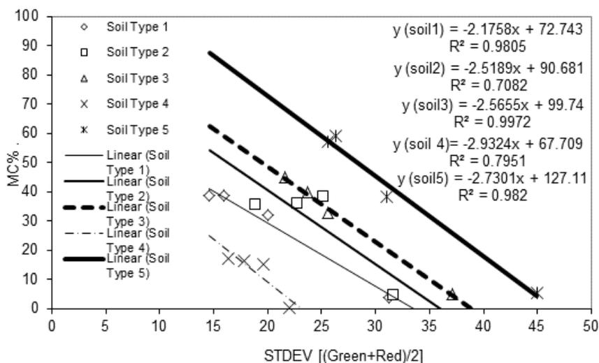
Figure 7. Moisture content (MC %) vs. average standard deviation of the green and red bands for the five soil types 1 (sand clay loam), 2 (clay loam), 3 (silty clay loam), 4 (sandy), and 5 (clayey) at the four moisture contents [air dried (a), FC (b), 1.5FC (c), and 2.0FC (d)] at 60-cm camera height.
