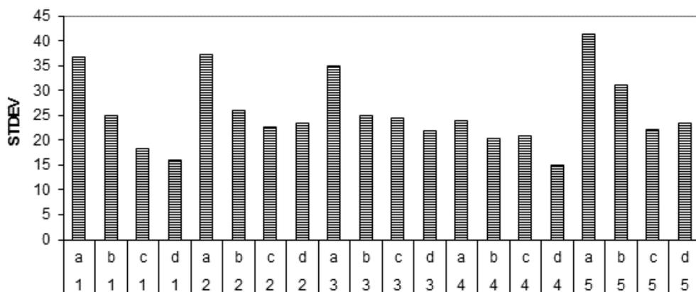
Figure 3. Average of the green and red standard deviations ( $ASD_{RG}$ ) for the five soil types 1 (sand clay loam), 2 (clay loam), 3 (silty clay loam), 4 (sandy), and 5 (clayey) at the four moisture contents [air dried (a), FC (b), 1.5FC (c), and 2.0FC (d)] at 30-cm camera height.
