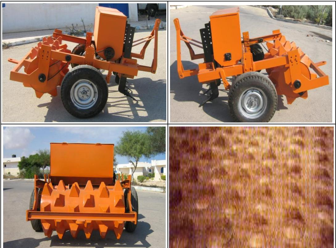
**Fig. 2: Photos of the manufactured combination machine and the experimental area with the mini reservoirs made by the machine**
