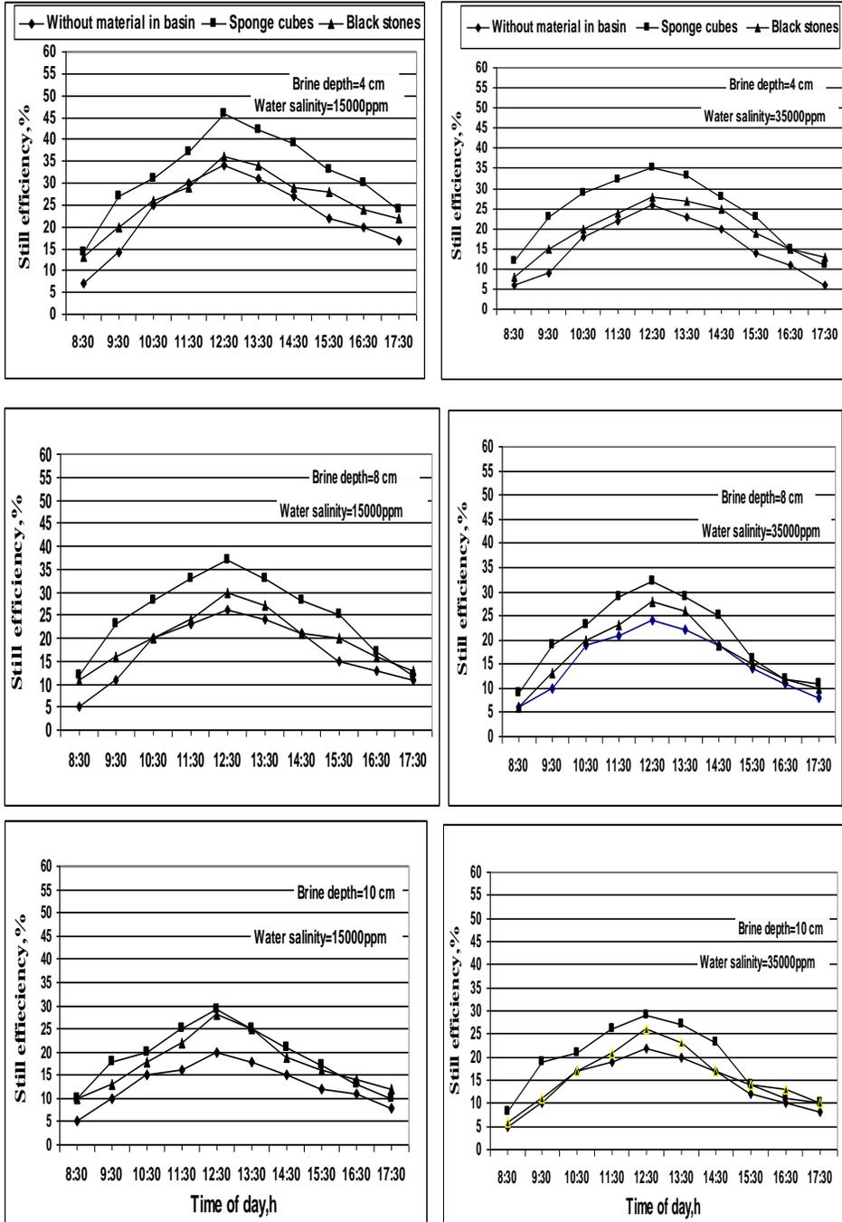
Fig.(6): Effect of brine depth , water salinity and the auxiliary black materials in basin on the still instantaneous efficiency during time of day.
