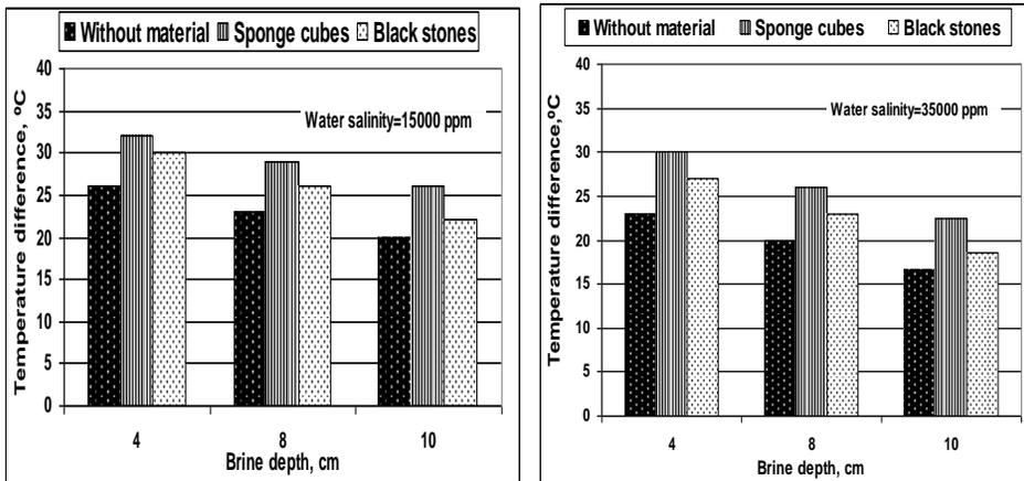
**Fig.(7): Maximum temperature difference between the glass cover and brine under the studied variables at noon hour.**
