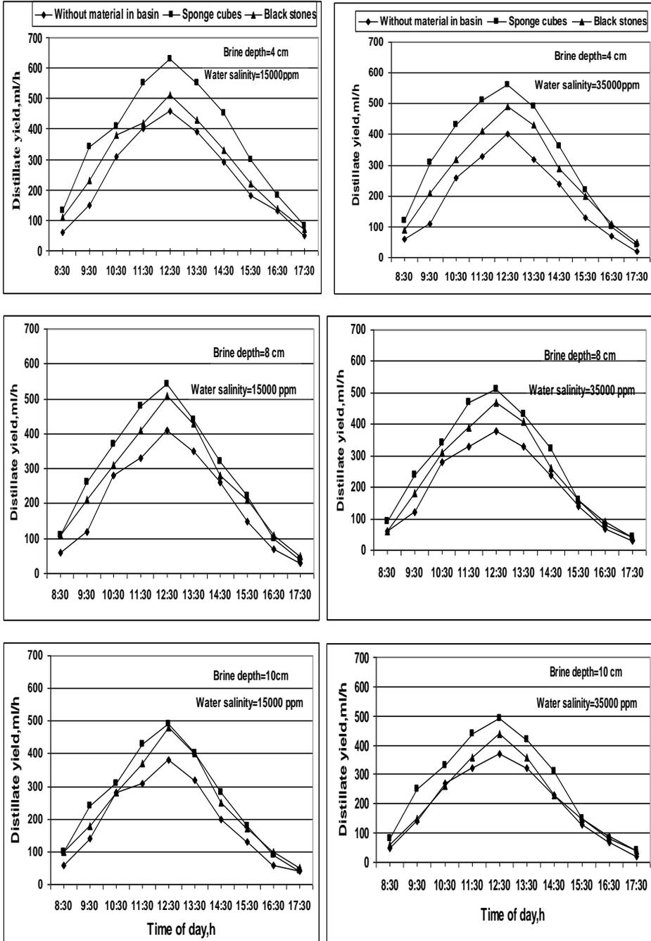
**Fig.(4): Effect of brine depth , water salinity and the auxiliary black materials in basin on the distillate yield during time of day.**
