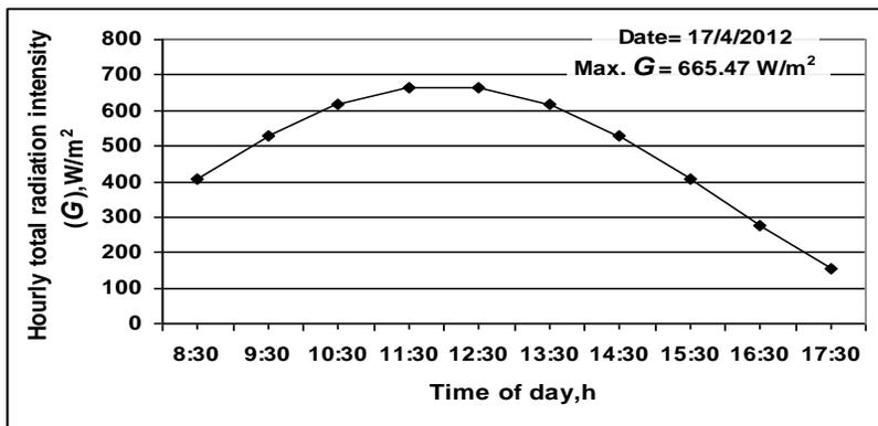
**Fig.(2): Hourly total radiation intensity distribution during the maximum hourly radiation day.**
