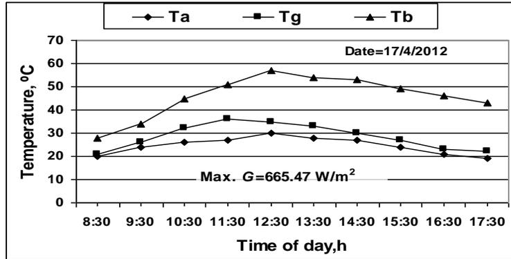
**Fig.(3): Variation of ambient temperature ( $T_a$ ), glass temperature( $T_g$ ) and brine temperature( $T_b$ ) during the day of maximum radiation.**
