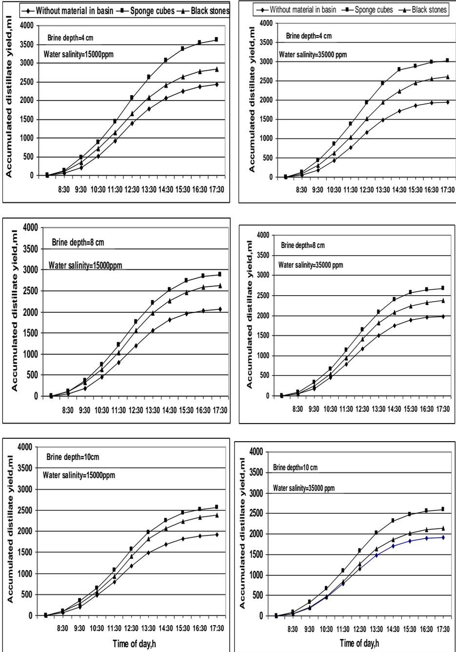
Fig.(5): Effect of brine depth , water salinity and the auxiliary black materials in basin on the accumulated distillate yield during time of day.
