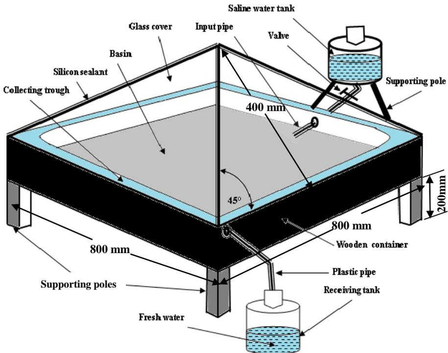
**Fig.(1): Schematic diagram of the pyramid-shaped solar still .**
