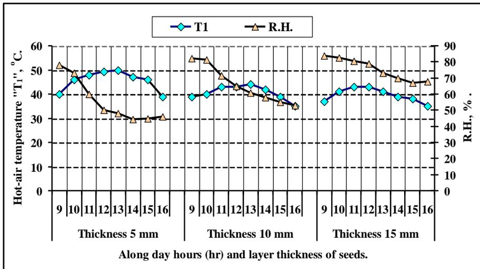
Fig. 5: Effect of drying time, layer thickness of cucumber seeds and drying hot-air temperature "T<sub>1</sub>" on relative humidity of air "R.H.".
