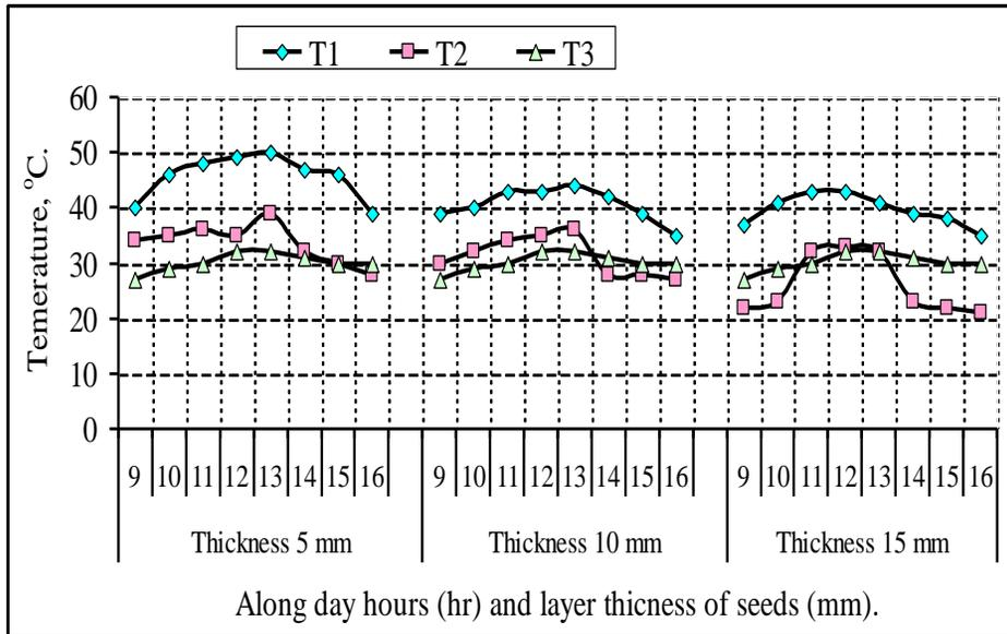
Fig. 4: Effect of drying time and layer thickness of cucumber seeds on the temperature (T<sub>1</sub>: hot-air temperature, T<sub>2</sub>: cucumber seeds temperature and T<sub>3</sub>: ambient temperature).
