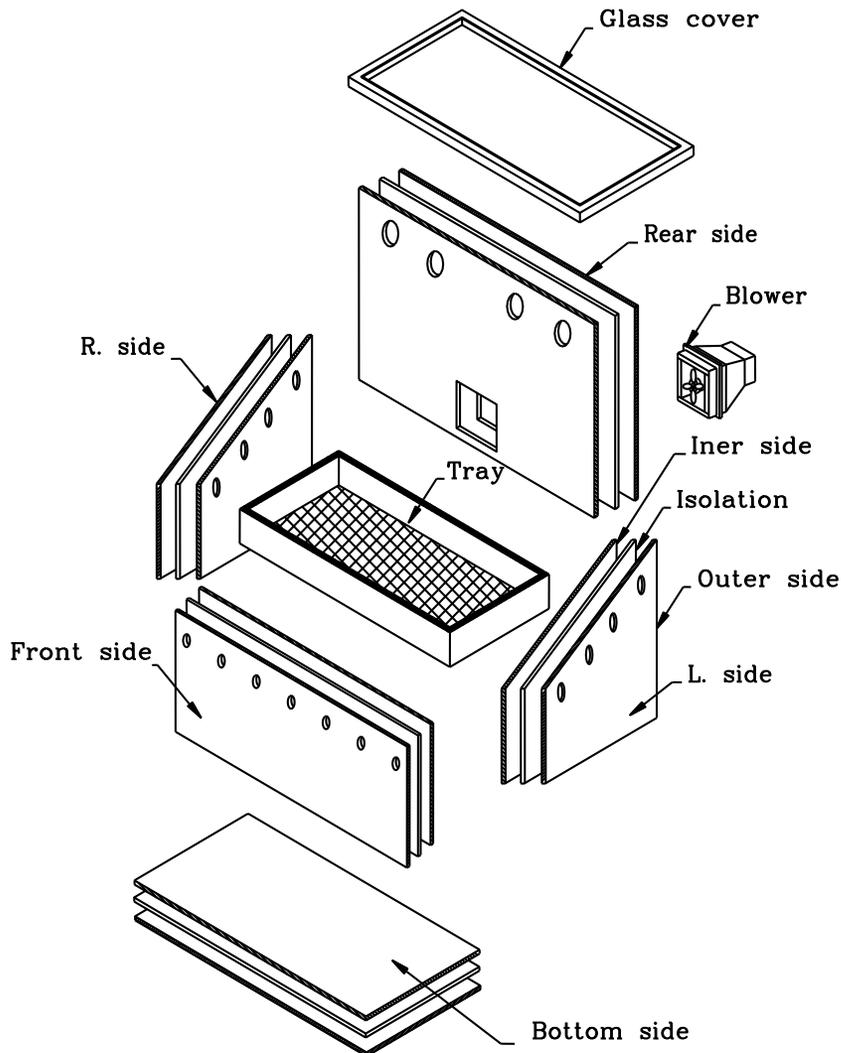
**Fig. 2: Isometric and parts of the cabinet dryer.**
