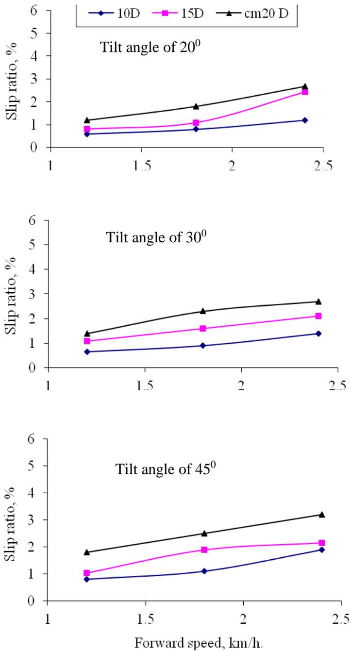
Fig. 9: Effect of forward and compressed wheel depth (D) on tractor wheel slip under different tilt angles, degrees for surface mulch
