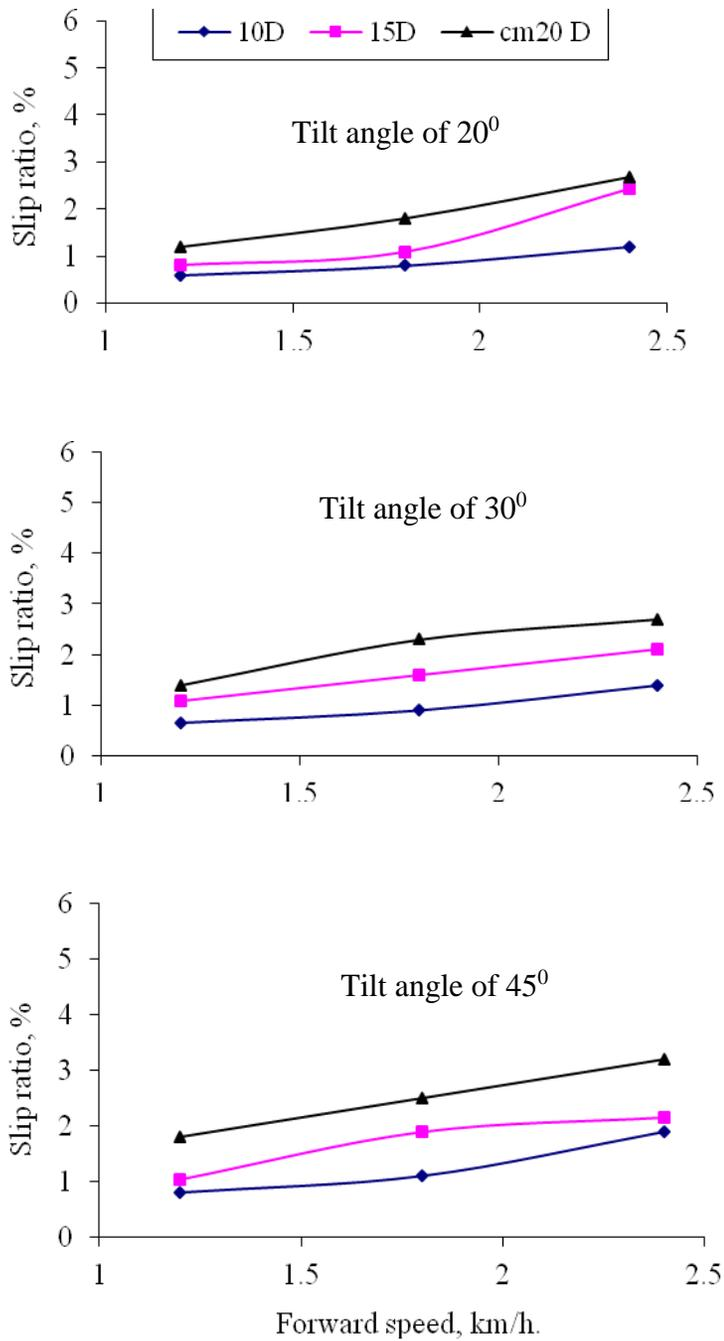
Fig. 8: Effect of forward speed and compressing-wheel depth, (D) on tractor wheel slip under different tilt angles for subsurface mulch
