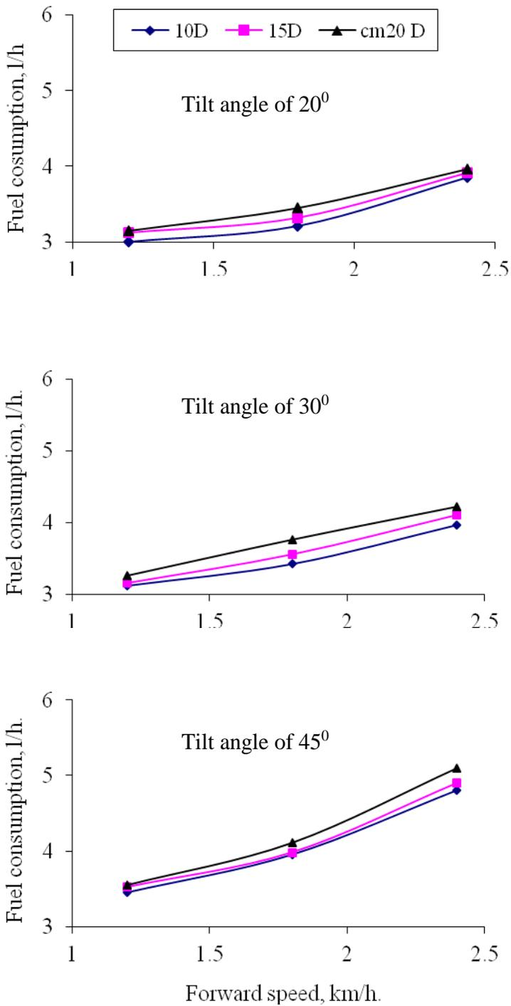
Fig. 11: Effect of forward speed and compressed wheel depth (D) on fuel consumption under different tilt
