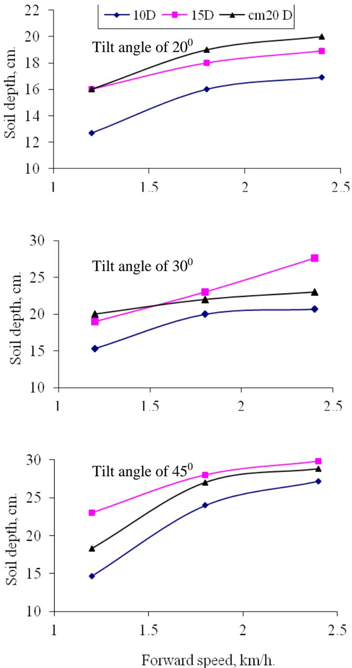
Fig. 7: Effect of forward speeds and compressing-wheel depth (D) on soil covering depth under different tilt angles for subsurface mulch
