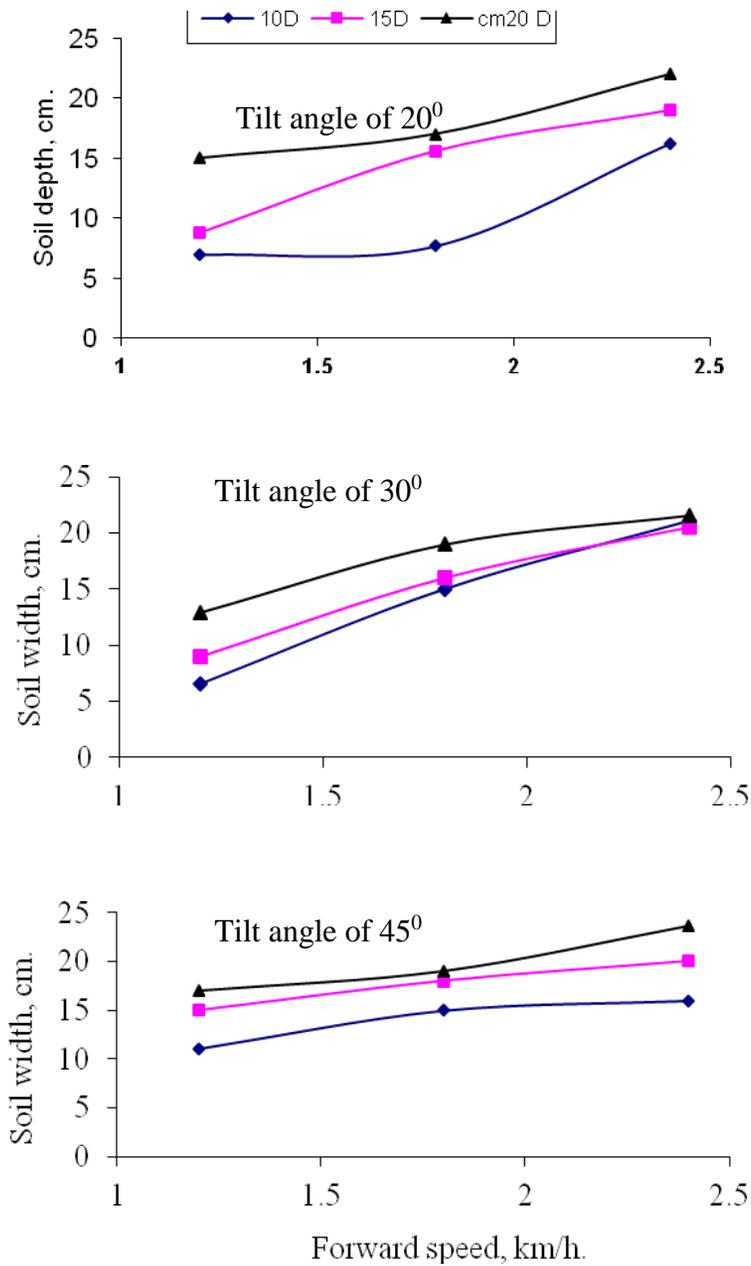
Fig. 12: Effect of forward speed, km/h on soil covering width, cm under different tilt angles, degrees for surface mulch
