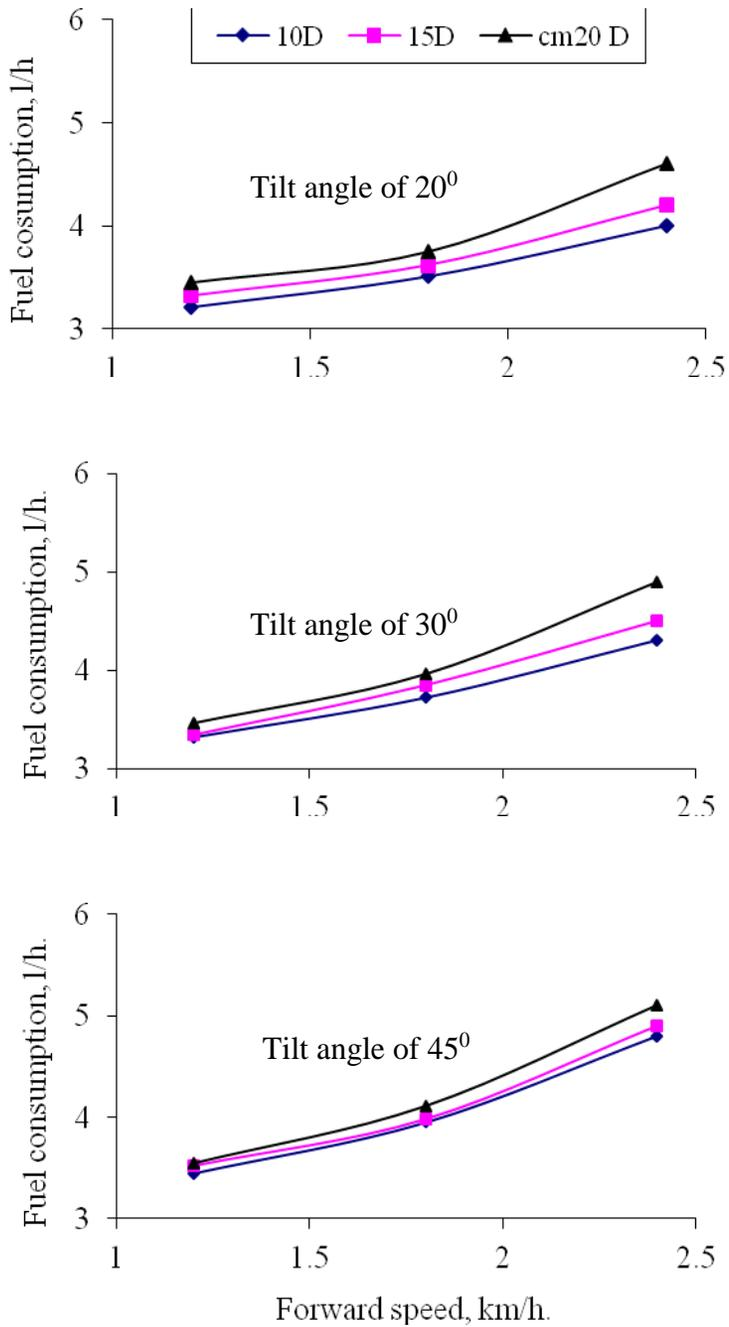
Fig. 10: Effect of forward speed and compressed wheel depth (D) on fuel consumption under different tilt angles for subsurface mulch
