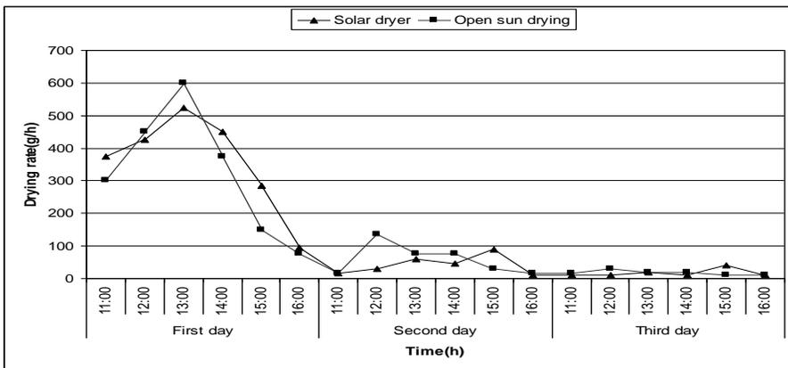
Figure( 7) Variation of drying rate with drying time of mint in solar dryer and open sun .
