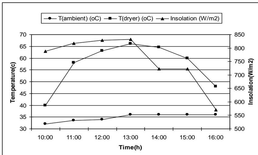
Figure (3) The variation of temperature in the dryer, ambient temperature and solar radiation intensity during (15 / 9 / 2013)
