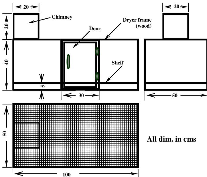
Figure (1): Schematic diagram of the solar dryer.
