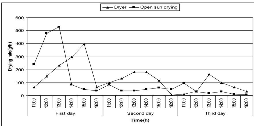
Figure(8) Variation of drying rate with drying time of grapes in solar dryer and open sun .
