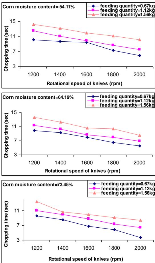
Fig (2): Chopping time at different levels of rotational speed of knives and different levels of dry feeding quantity for modified chopping machine
