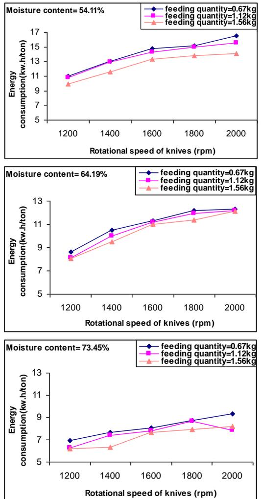
Fig(8): Chopping energy at different levels of rotational speed of knives and different levels of dry feeding quantity at the three levels of moisture content for the modified machine.
