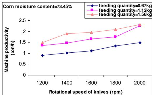
Fig(10): Machine productivity at different levels of rotational speed of knives and different levels of dry feeding quantity at the three levels of moisture content for the modified machine
