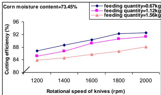
Fig(6): Cutting efficiency at different levels of rotational speed of knives and different levels of dry feeding quantity at the three levels of moisture content for the modified machine.
