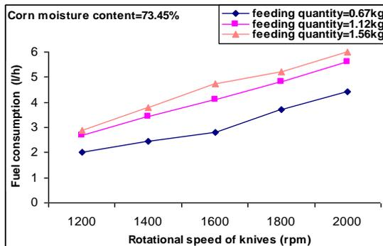
Fig (4): Fuel consumption at different levels of rotational speed of knives and different levels of dry feeding quantity for modified machine
