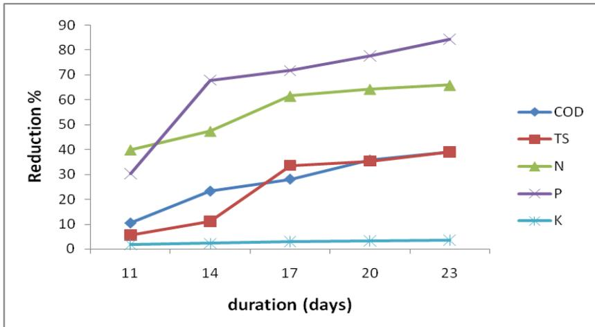
Fig. 4: The pollution reduction for 2.5kg/m<sup>2</sup> seed quantity and 3days water time duration.
