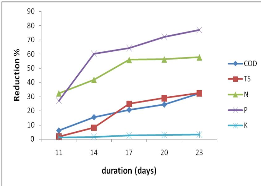
Fig. 2: The pollution reduction for 1.5kg/m<sup>2</sup> seed quantity and 3days water time duration.
