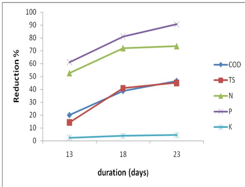
Fig. 5: The pollution reduction for 2.5kg/m<sup>2</sup> seed quantity and 5days water time duration.
