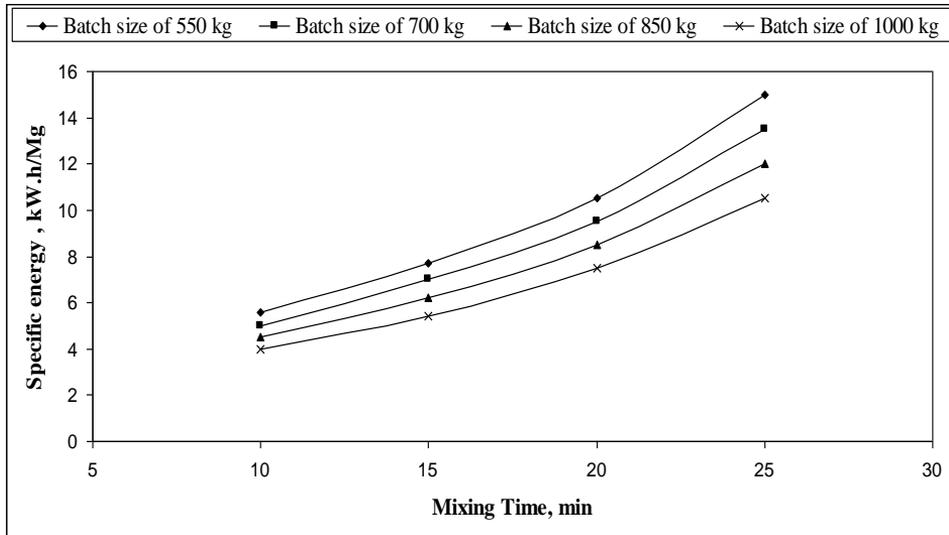
**Fig. (6): Effect of mixing time and batch size on specific energy**
