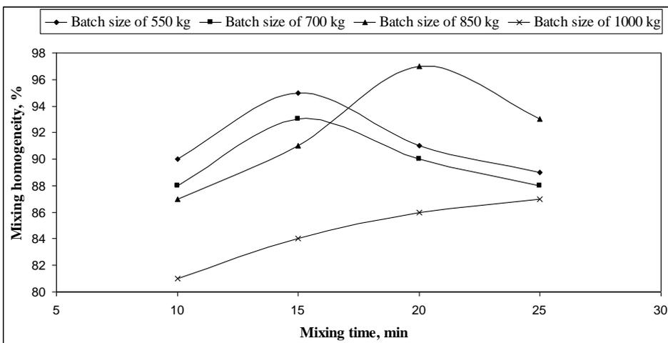
**Fig. (4): Effect of mixing time and batch size on the mixing homogeneity**
