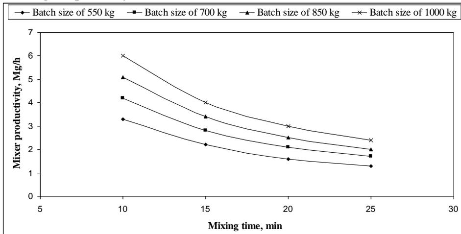
**Fig. (5): Effect of mixing time and batch size on mixer productivity**
