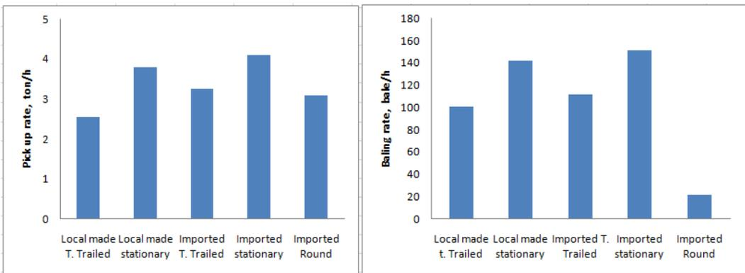
Fig (1) Pick-up rate and baling rate of the locally made VS imported balers
