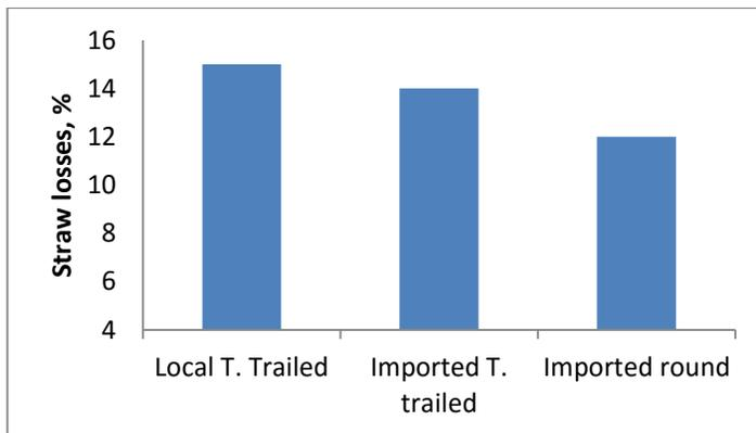
Fig (2) straw losses (unpicked straw) of the tractor pulled balers
