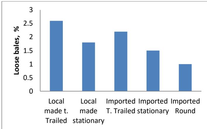
Fig (4) percent of loosen bales of the locally made VS imported balers
