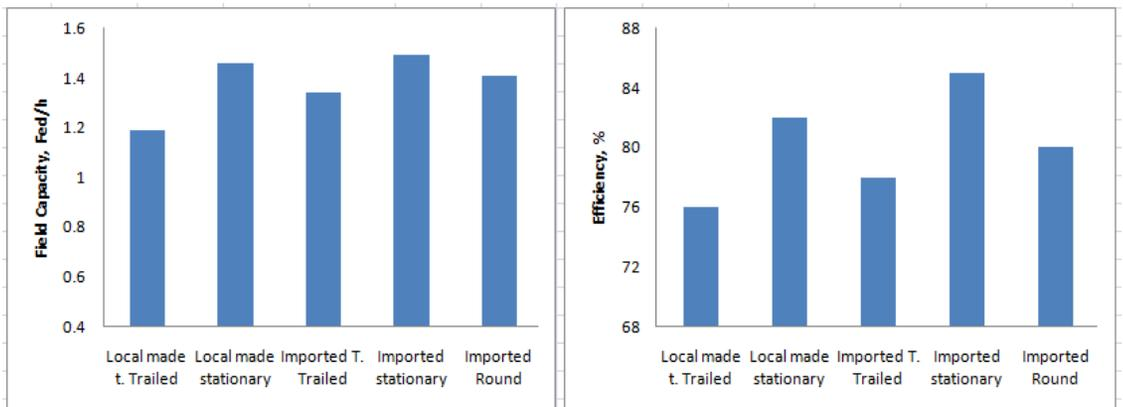
Fig (5) Field capacity and efficiency of locally made vs imported balers
