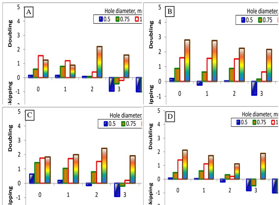
Figure (10): The effect of both feeding device height and orifice diameter on seeds skipping and doubling
