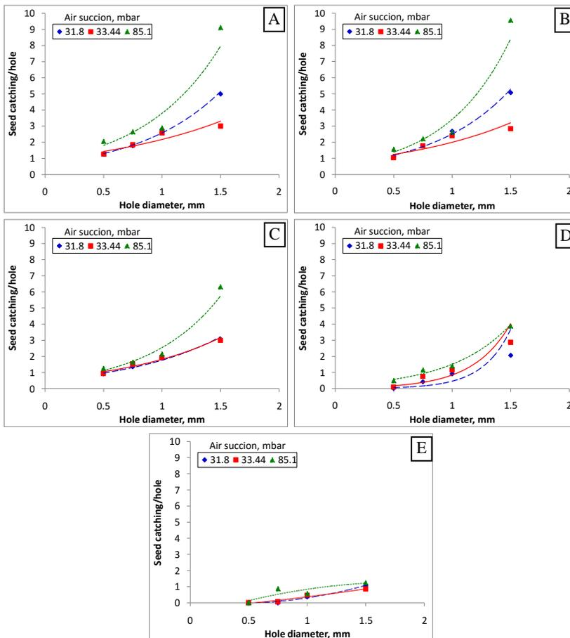
Figure (9): Effect of air pressure suction on tomato seeds catching
