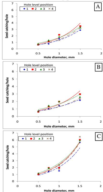
**Figure (8): Effect of orifice diameter on tomato seeds catching at different orifice level position**
