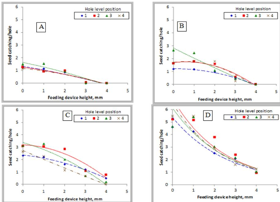
Figure (6): Effect of feeding device height on tomato seeds catching at suction tube orifice diameter of 1.5 mm.
