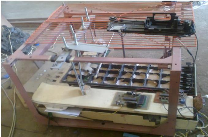
Figure (1): General view of the developed precision seeder
