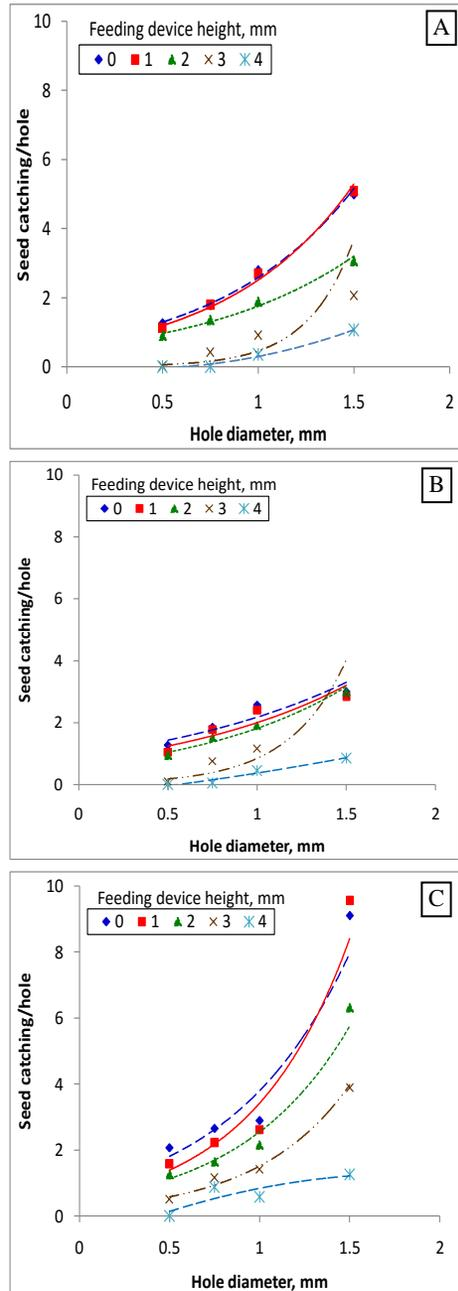
Figure (7): Effect of orifice diameter on tomato seeds catching at different feeding device height
