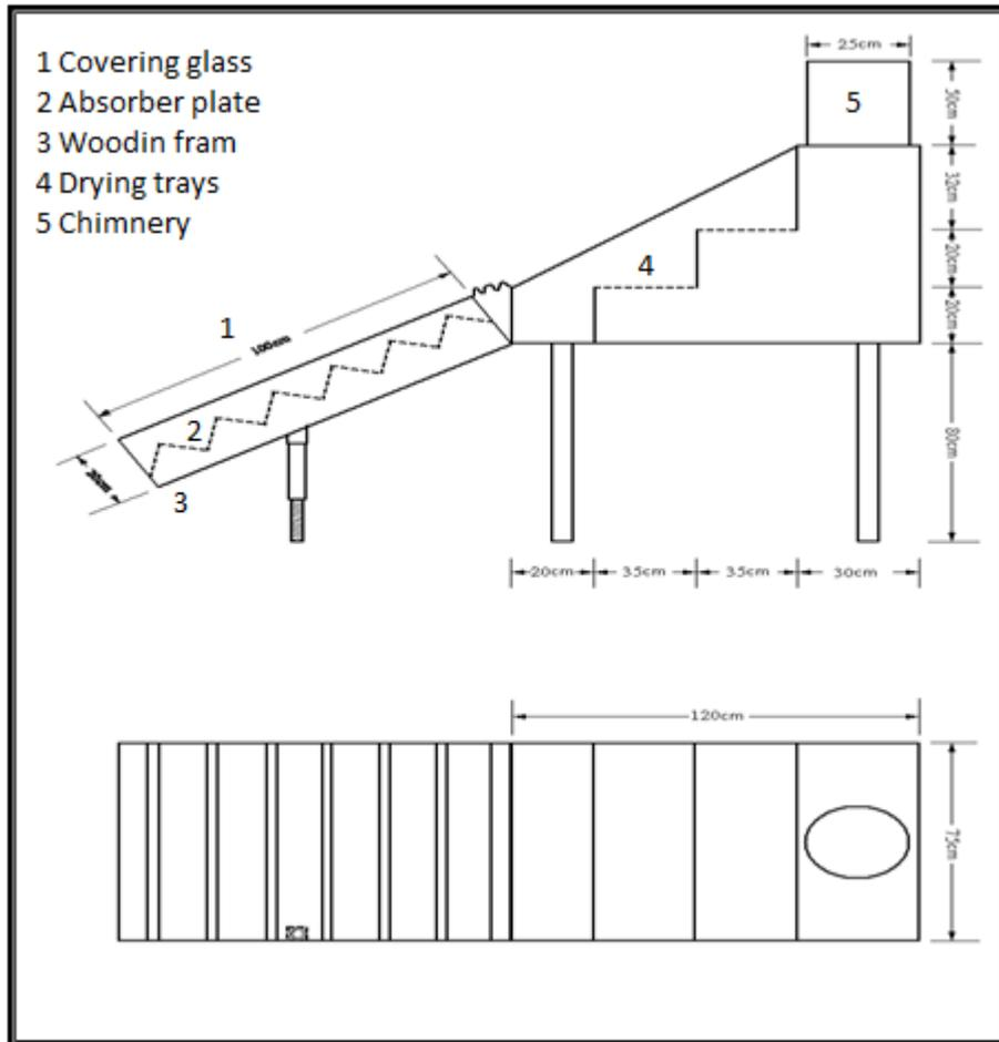
**Fig. (1): Schematic diagram of solar drier.**
