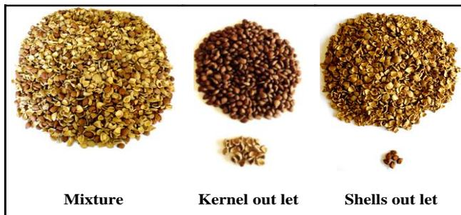
Fig. (7): Result of separation process.
