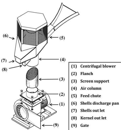
Fig. (3): Assembling of separation unit.
