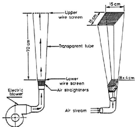
Fig. (4): Terminal velocity apparatus (Awady and El-sayed, 1994).
