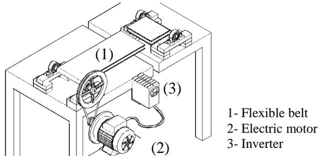
Fig. (5): Feeding rate measurement apparatus.
