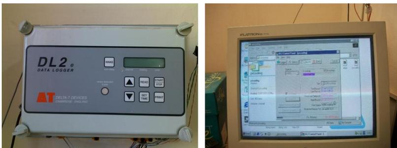
**Fig. 3.** Data logger DL2 version 5.0 connect with PC
