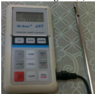
**Fig. 4.** Air velocity meter and its probe.
