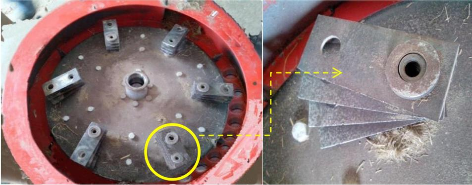
**Fig.2 Cutting and crushing unit with blades sets.**
