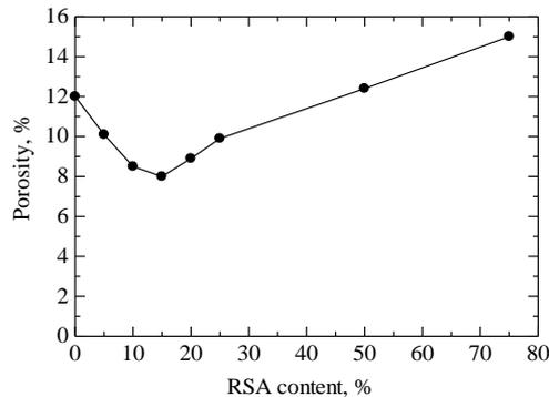
**Fig. 10.** Variation of OPC-RSA mortars porosity at 28 days
