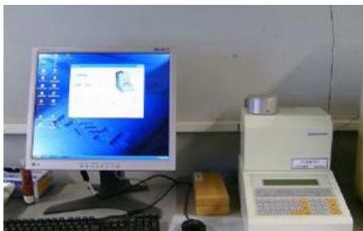
**Fig. 4.** Helium pycnometer device to measure the true density
