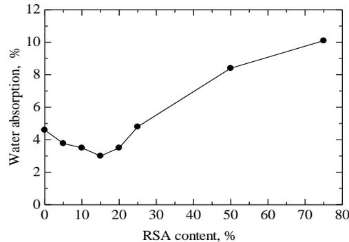
**Fig. 11.** Variation of OPC-RSA mortars water absorption at 28 days
