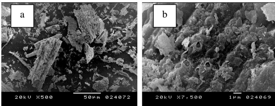
**Fig. 8.** (a) SEM images of RSA particles, and (b) SEM image of RSA particle surface
