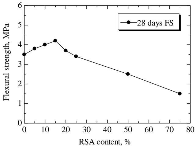
**Fig. 14.** Variations of flexural strength at different percentages of RSA.
