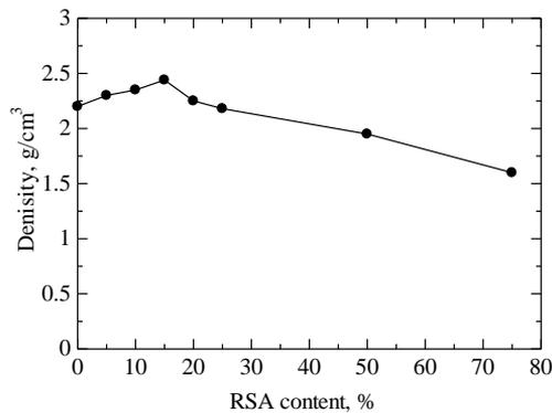
**Fig. 9.** Variation of OPC-RSA mortars densities at 28 days
