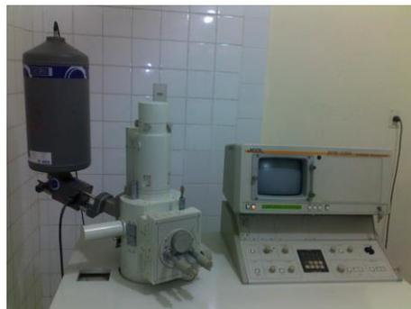
**Fig. 3.** JSM-5300 Scanning microscope
