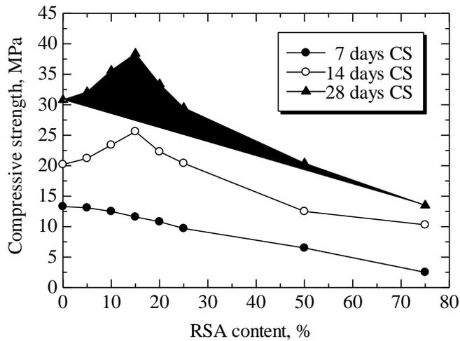
**Fig. 13.** Variations of compressive strength at different percentages of RSA.
