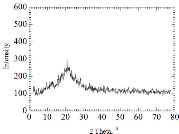
**Fig. 7.** The X-ray spectrum of RSA.
