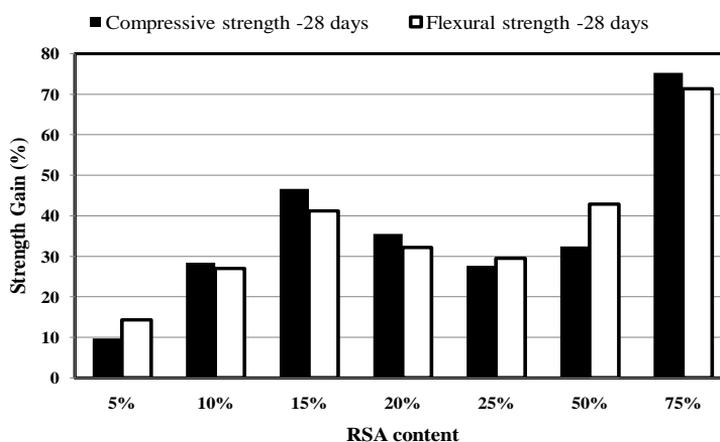
**Fig.16.** Strength gain (SG) for OPC-RSA mortars at 28 days.
