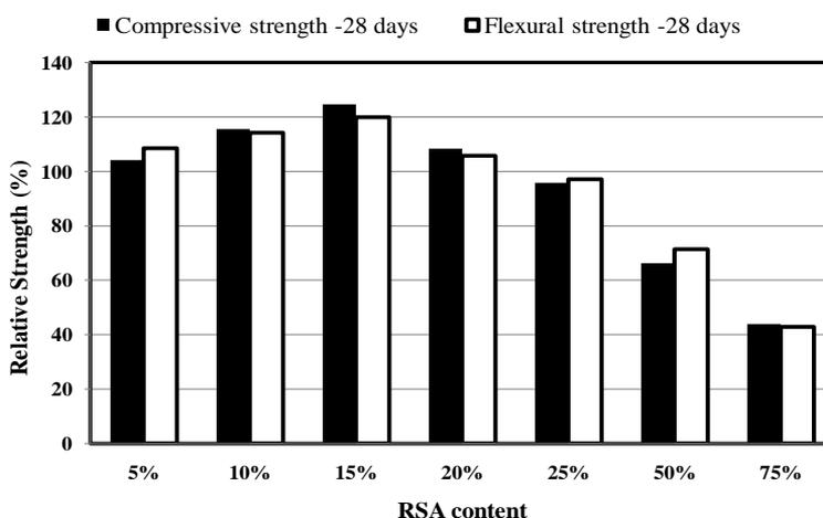
**Fig.15.** Relative strength (RS) for OPC-RSA mortares at 28 days.
