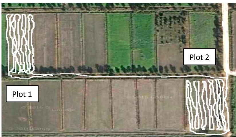
Fig.(6). The track of the tractor in the field without guiding by GPS.
