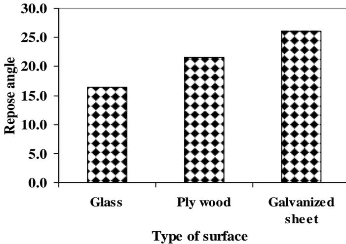
**Fig.(6): Angle of repose for date fruits on different material surface.**
