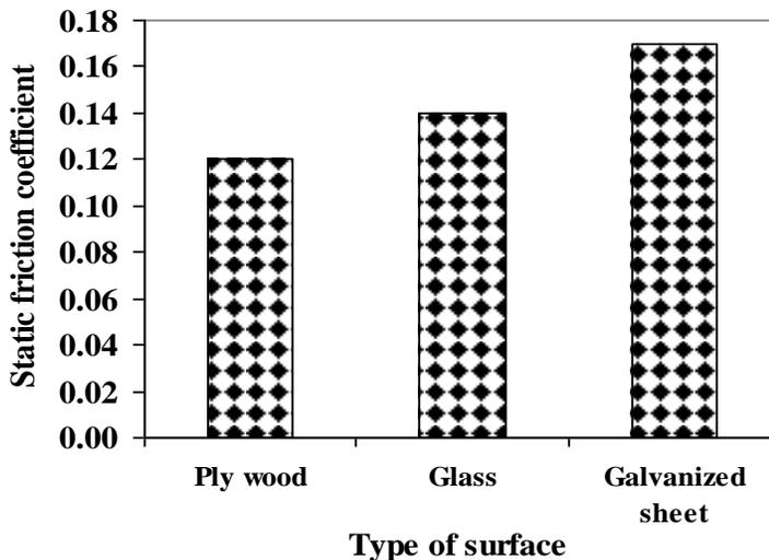
**Fig. ( 7 ):Static friction coefficient for date fruits on different material surface.**
