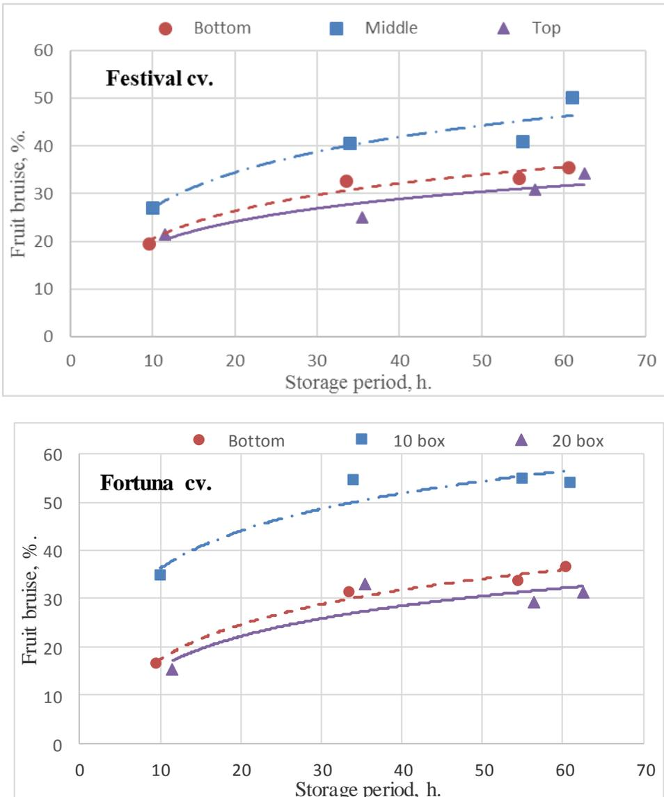
**Fig. 7: Effect of storage period after the vibration treatment on the fruit bruise at different box positions on vibrational table.**
