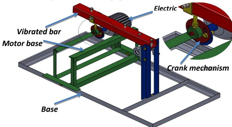
Fig. 2: All parts of mechanism as assembly.
