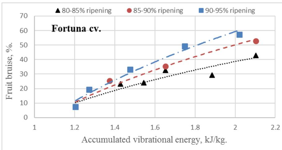
**Fig. 5: Effect of energy spectral density on the fruit bruise at different fruit ripening degrees.**
