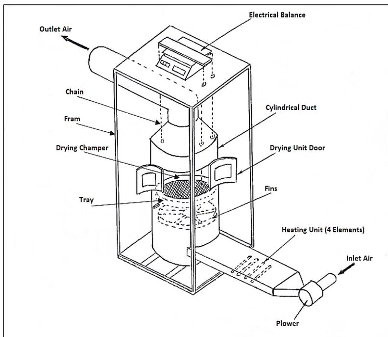
**Fig. (1): Schematic diagram of the experimental dryer.**
