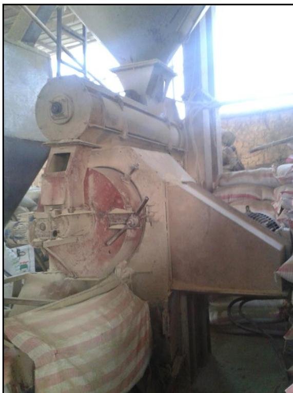
Fig. (2): The ring die animal feed pellets extruder.
