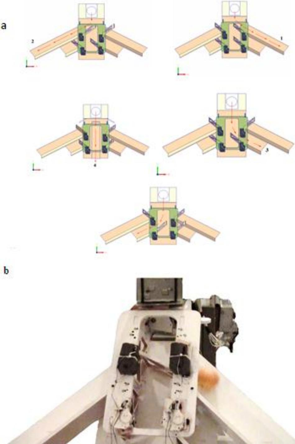
**Fig. 3 a: Schematic view and b: photograph of arrangements of grading gates and grading paths**
