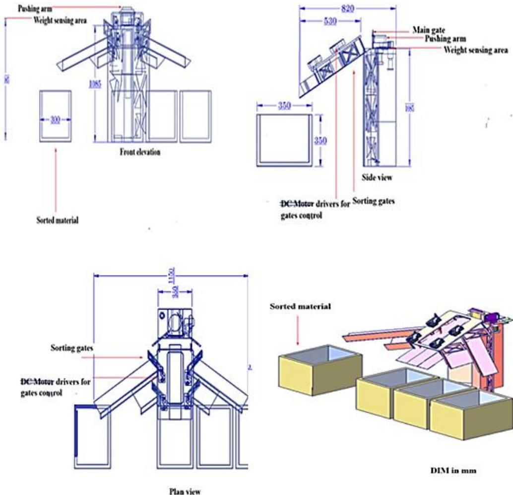
**Fig. 2 Sketch for weight and grading unit**
