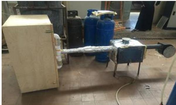
**Fig. (1). Photo of the biogas dryer**
