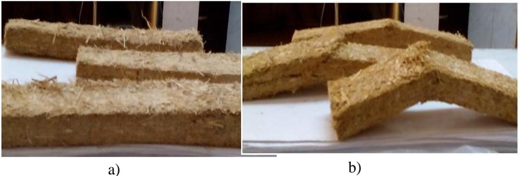
Fig. 1: samples for static bending test, a) before the test. b) after the test.
