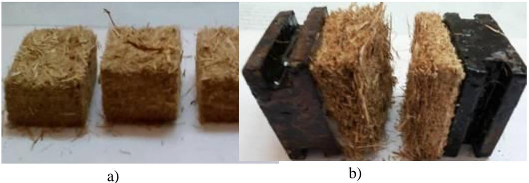
Fig. 2: samples for tension test, a) before the test. b) after the test.
