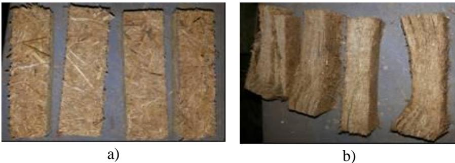
Fig. 3: Compressive strength test samples, a) before the test. b) after the test.
