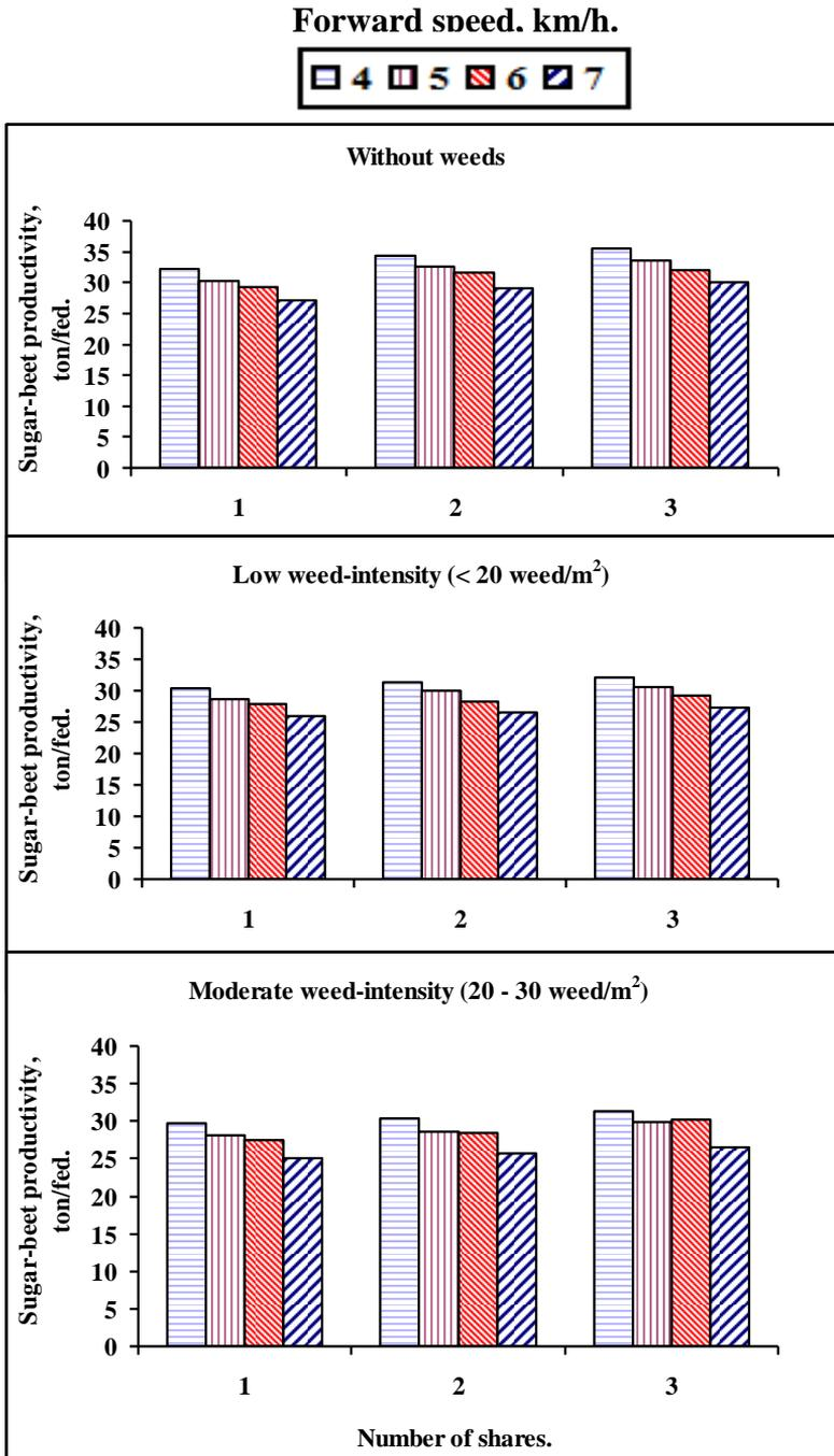
Fig. 6: Effect of forward speed, number shares on sugar-beet productivity without weed, at low and moderate weed intensity.
