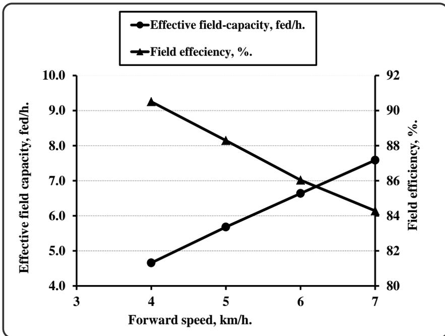
Fig. 9: Effect of forward speed on effective field-capacity and field efficiency of inter-row cultivator.
