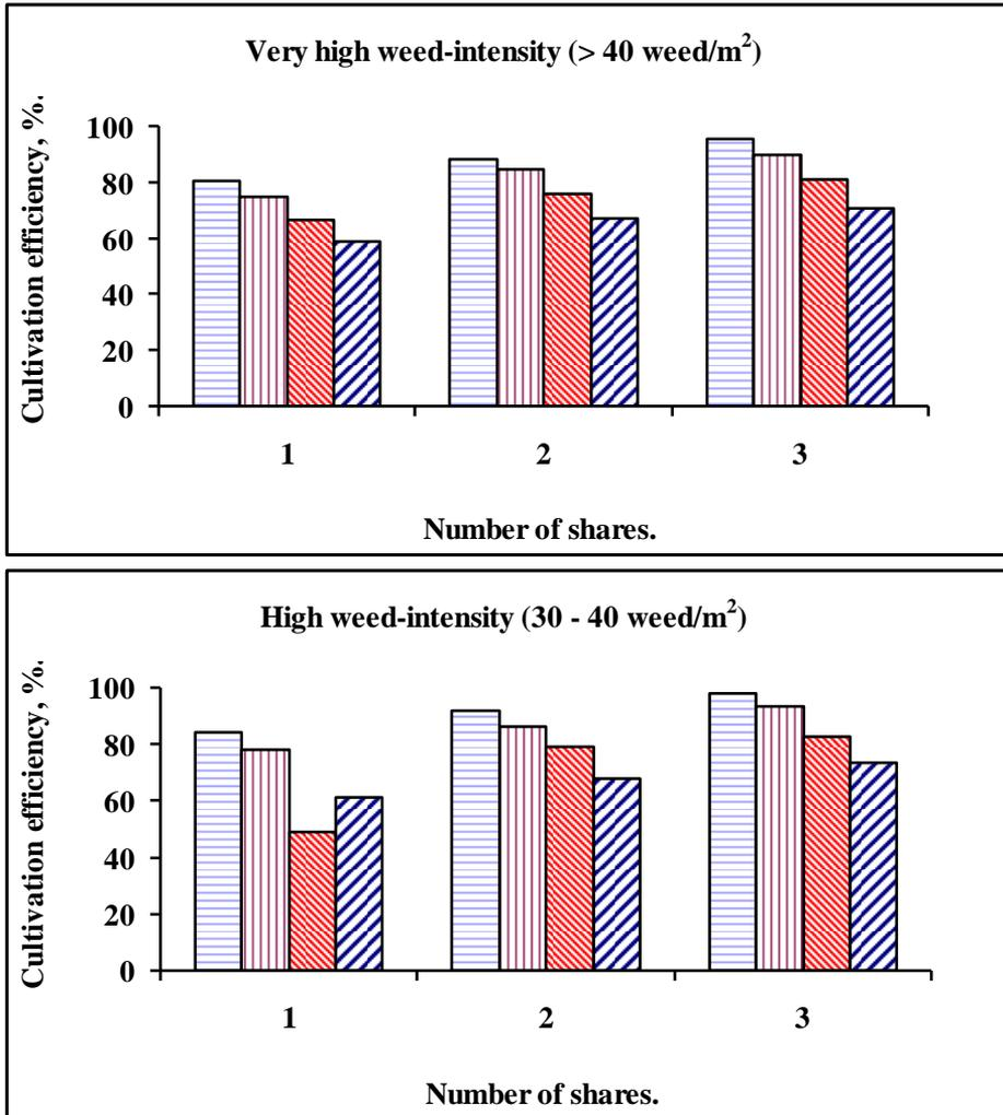
Fig. 4: Effect of forward speed, number shares on cultivation efficiency at high and very high weed intensities.
