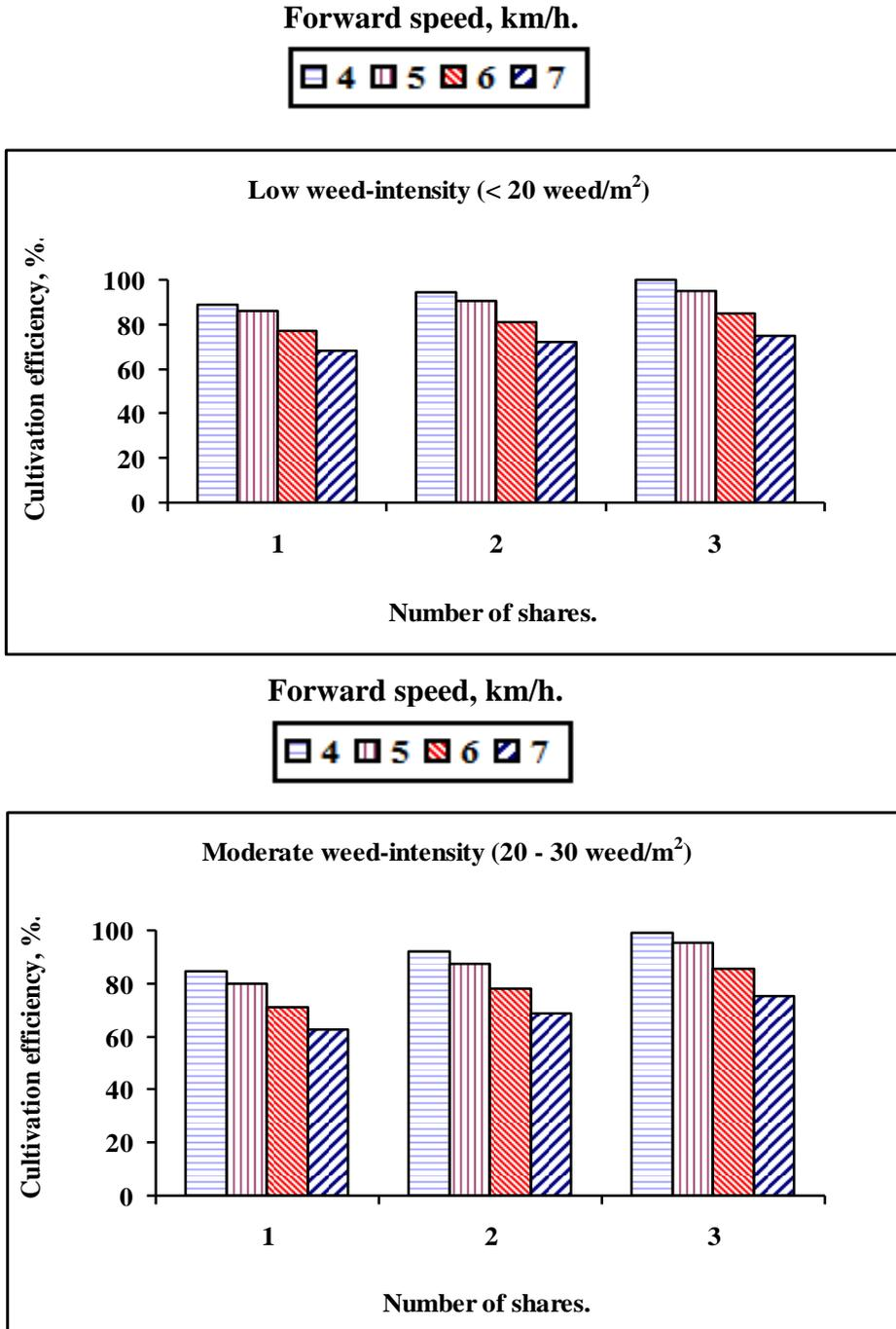
Fig. 3: Effect of forward speed, number shares on cultivation efficiency at low and moderate weed intensities.
