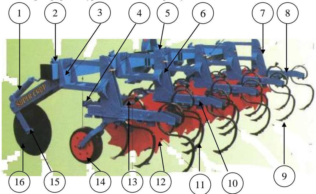
Fig. 1: The tested precision inter-row cultivator.
