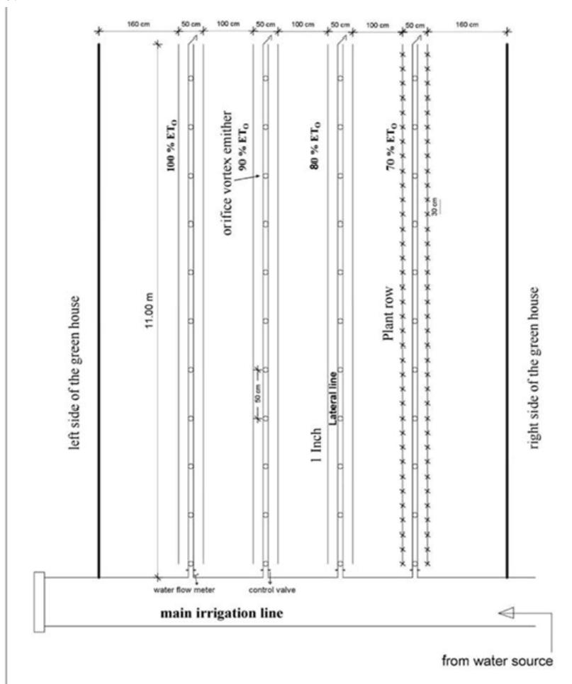
**Fig. 1: Schematic diagram of surface drip irrigation system and the studied tested treatments for each greenhouse.**
