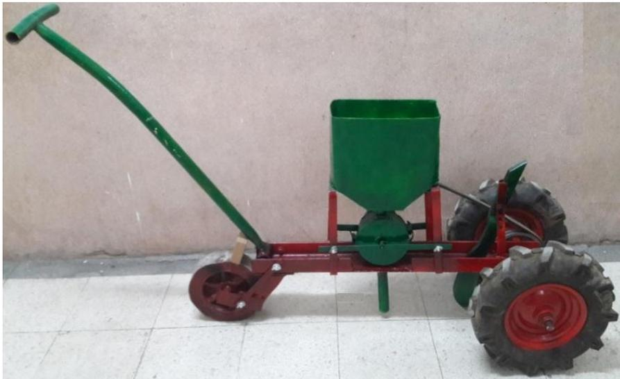
**Fig (3): Photo of the designed manually operated single row planter**
