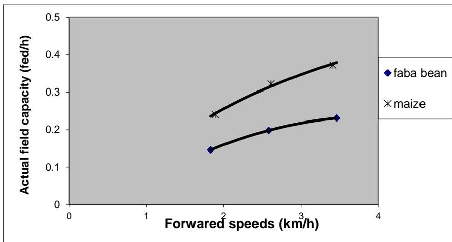
**Fig. (12): Effect of different forward speeds on actual field capacity.**
