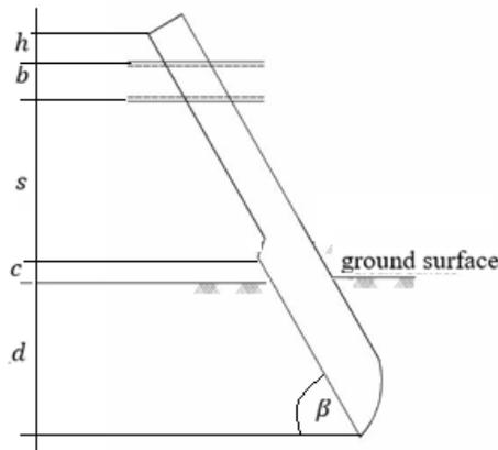
Figure 9. The main dimensions of the furrow opener
