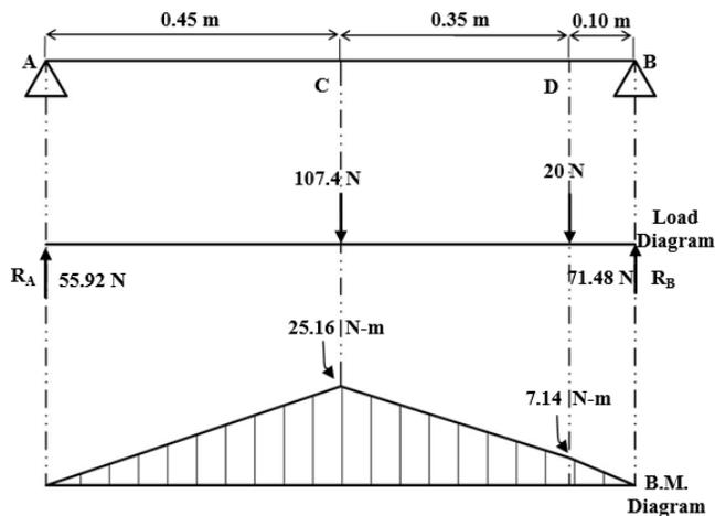
**Fig. (7): The bending moment diagrams of the main frame beam**
