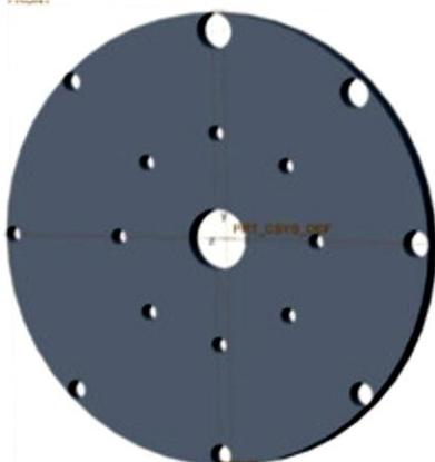
**Fig. 1. View of a plate type seed-metering device for the planter**
