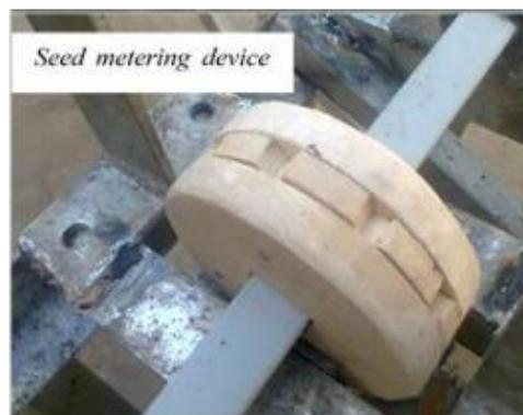
**Fig. 2. Photograph of seed-metering of maize planter**
