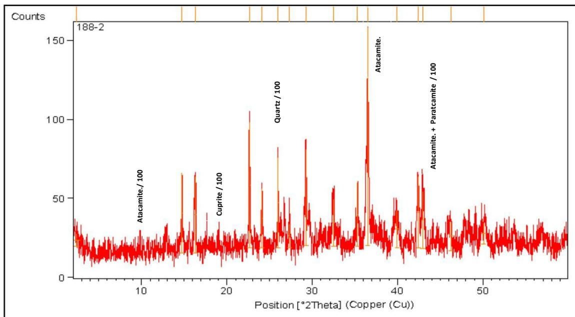
Fig. 10 Shows XRD pattern of corrosion sample for bronze works.
