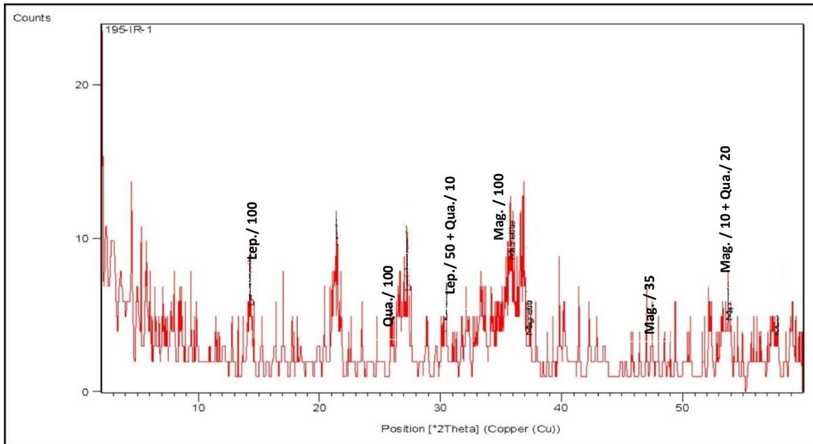
**Fig. 11 Shows XRD pattern of corrosion sample of the iron table.**
