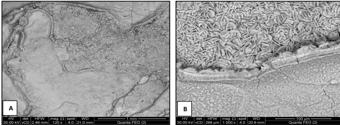
**Fig. 7 A, B, shows cracks, breaks, erosion and layers of rust from the microscopic images of the scanning electron microscope of the iron table.**
