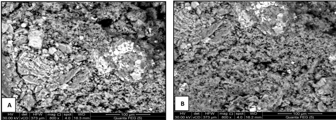
**Fig. 8 A, B, Shows the layers of corrosion compounds, cracks and mineral grains through the microscopic images of the scanning electron microscope for bronze artifacts**
