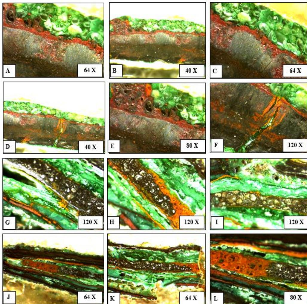
Fig. 6 A-L, shows cracks, erosion and layers of corrosion products in different colors with iron through the stereoscopic examination of the iron table samples.
