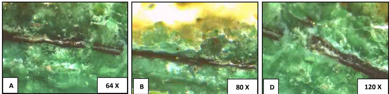
Fig. 5 A, B, C, shows the layers of corrosion products with the bronze alloy through the stereo microscope examination of the bronze artifact's samples.
