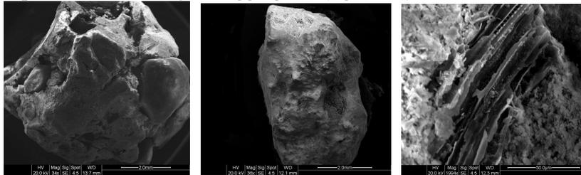
Figure 4: SEM images showing left: weak contacts between rounded grains and the binder, middle: stronger contact with scoria, and right good adheres of lime binder to organic straws.
