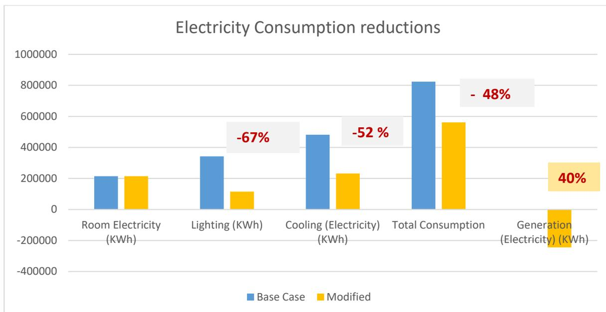
**Table (10)** Reductions in Lighting, Cooling load and total consumption.
