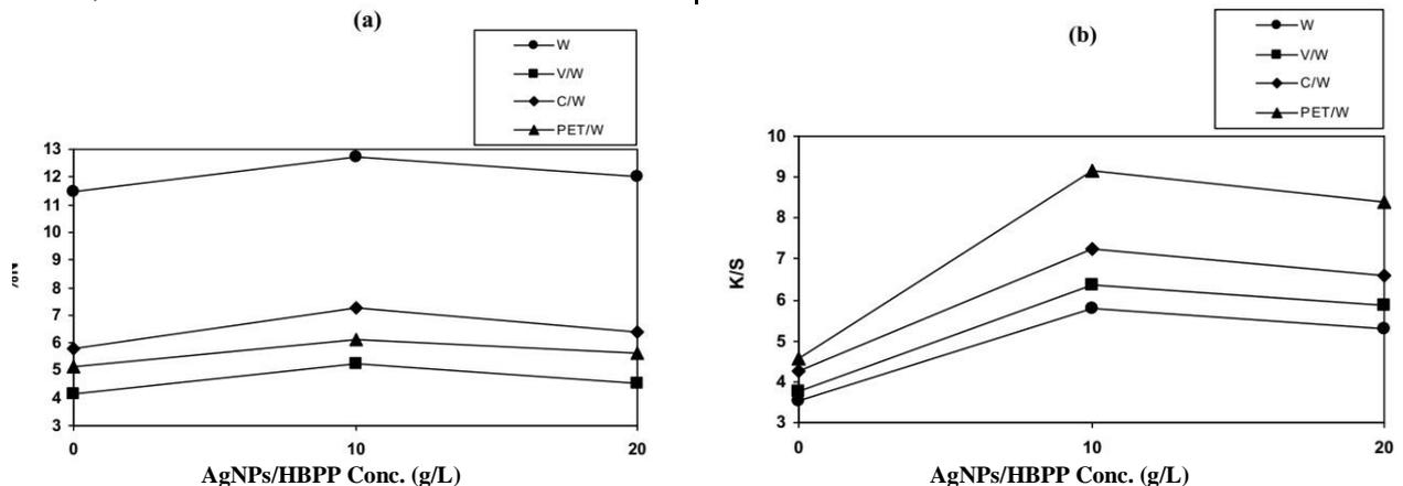
Fig 2. Effect of post-treatment of the W: wool, V/W: viscose/Wool, C/W: cotton/wool and PET/W: polyester/wool printed fabric samples with AgNPs/ HBPAA composite on (%N, a) and (K/S, b) val
