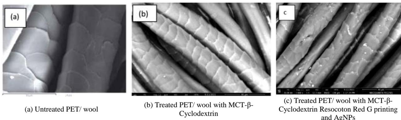
Fig 8. SEM image of untreated PET/ wool (a). treated PET/wool with MCT- $\beta$ -Cyclodextrin (b). treated PET/wool with MCT- $\beta$ -Cyclodextrin/ Resocoton Red G printing and AgNPs post- treated (c)
