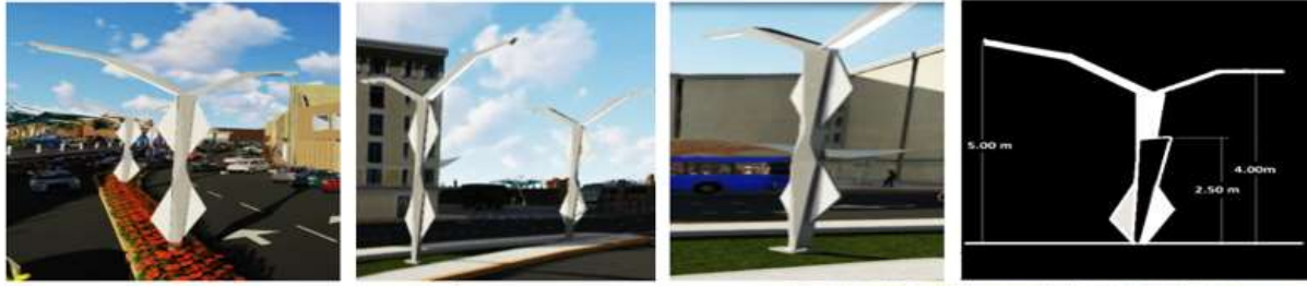
Fig.16- (1-2): The lighting units were designed in a simple way to suit the design of the place where it works with a hybrid energy system, using electricity in addition to panels and solar cells for the optimal use of sunlight in the area.
