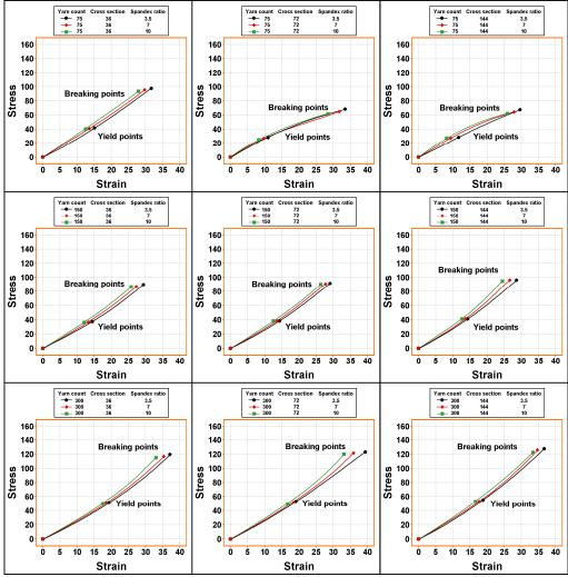
Fig. (7): Stress-strain curves of spandex/polyester woven fabrics as affected by the interaction effect among yarn count, cross section and spandex ratio.
