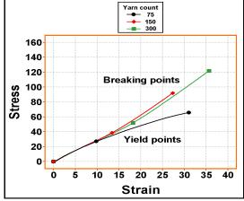
Fig. (8): Stress-strain curves of spandex/polyester woven fabrics as affected by yarn count.
