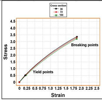
**Fig. (2): Stress-strain curves of spandex/polyester spun yarn as affected by yarn cross section.** The effect of three spandex ratios (3.5, 7 and 10 %) on tensile and elongation behaviors of spandex/polyester yarns are tabulated in Table (3) and diagrammed plotted in stress-strain curves as shown in Fig. (3). **Here are an elongation behaviors of spandex/polyester yarns are tabulated in Table (3)** and diagrammed plotted in stress-strain curves as shown in Fig. (3).
