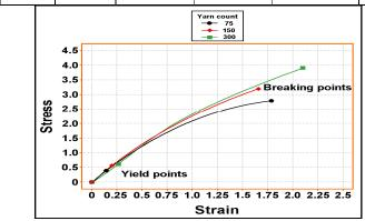
Fig. (1): Stress-strain curves of spandex/polyester spun yarn as affected by yarn count.
