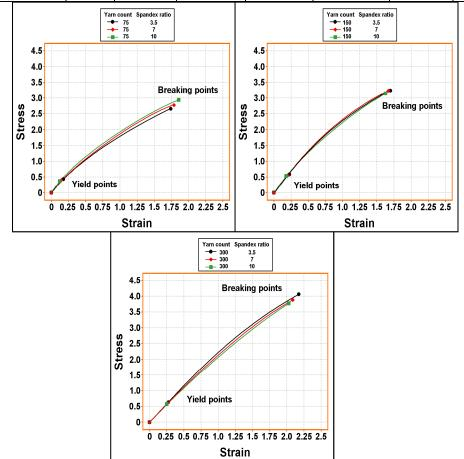
Fig. (5): Stress-strain curves of spandex/polyester spun yarn as affected by the interaction effect between yarn count and spandex ratio.
