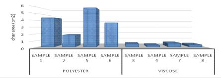
Fig. (9) Relationship between weft materials and flame resistance
