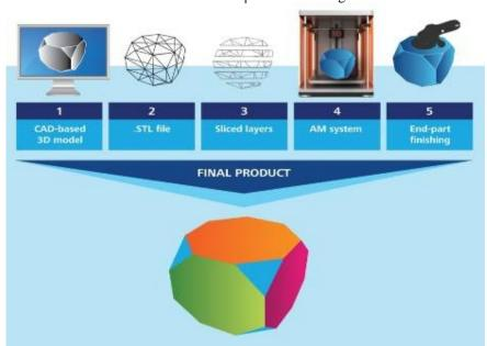
Figure (1) 3d printing process - Source: (Mark Cotteleer- 2014)
