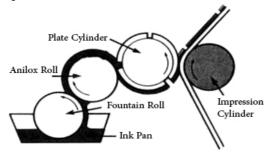
Figure 1: Flexographic Printing Process Source: (http://www.brobygrafiska.sewpcontentuploads201302Anilox\_rolls)
