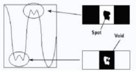
Figure 2a: Bars with voids and spots in the spaces
