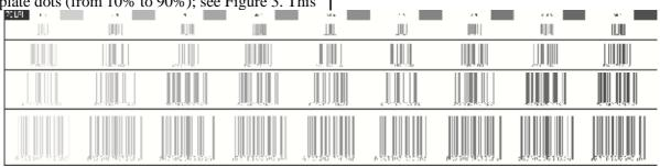
Figure 3: Barcodes with sizes scaled from 25% to 200% from the original one was printed in variable plate screens (from 70 lpi to 130 lpi) and plate dots (from 10% to 90%)
